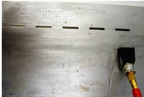
Figure 13 0.25"/10MHZ KBA Highly Damped Transducer with 60 Degree Wedge on the ETW Type II Calibration Plate
