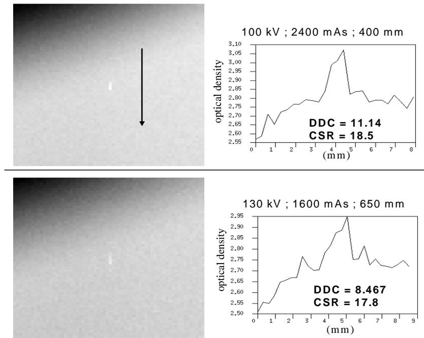
**Figure 7:** Simulated images for the optimal configuration (no scatter) and the usual configuration.
