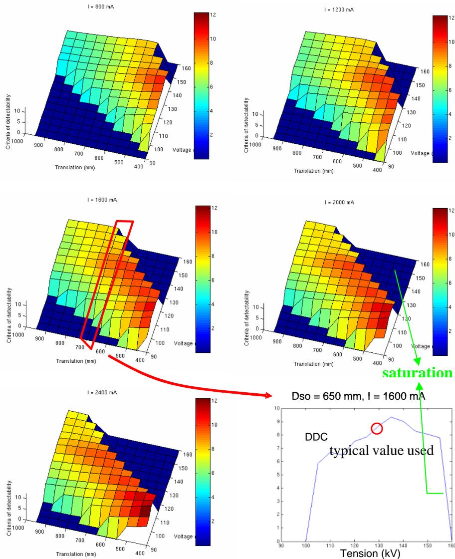
**Figure 6:** optimization surfaces get for the stiffener part inspected with the film M100 (no scatter simulation).
