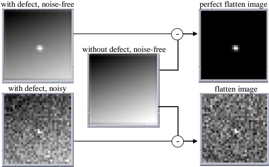
**Figure 2:** example of flattening process applied on noisy and noise-free images.
