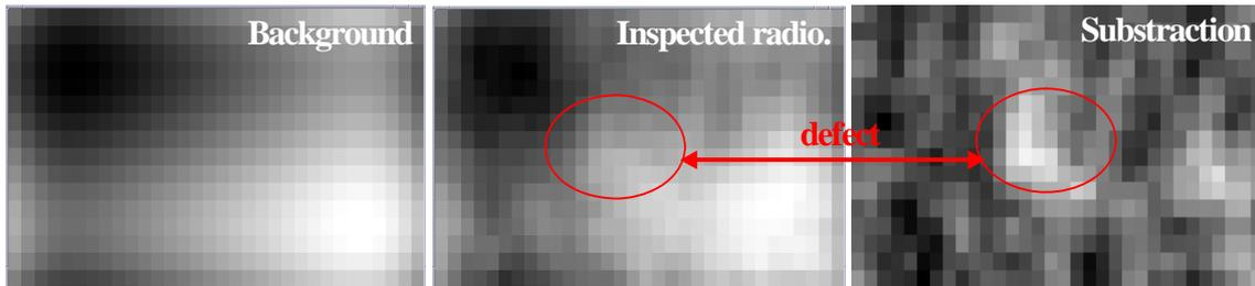
**Figure 4:** defect visibility on the inspected radiograph and the flatten one get by subtraction.
