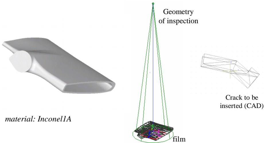
**Figure 5:** Radiographic inspection of the SNECMA stiffener part.
