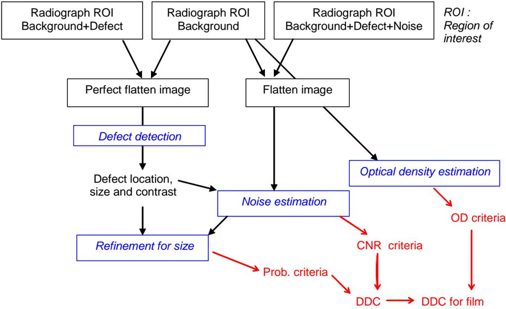
**Figure 3:** scheme for computing defect detectability criteria (*DDC*).
