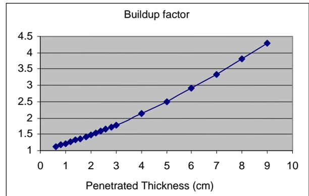
Fig. 5 Buildup factor calculated through simulation-configuration A2.
