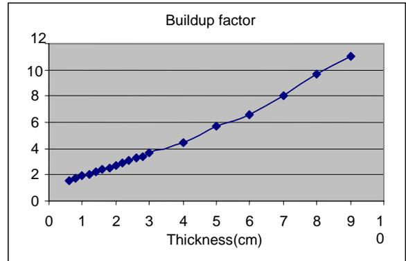
Fig. 3 Buildup factor calculated through simulation-configuration A1.
