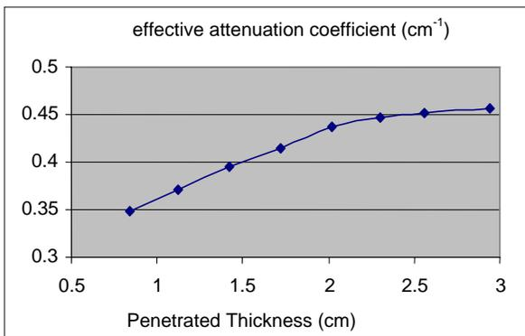
Fig. 6 Effective attenuation coefficient ( $\text{cm}^{-1}$ ) calculated through simulation- configuration A3.
