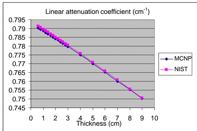
Effective attenuation coefficient ( $\mu_{\text{eff}}$ ) and buildup factor (B) are calculated by Monte Carlo simulation for A1 configuration. The results are illustrated in Figs. 2 and 3, respectively. The results of the same parameters are indicated on Figs. 4 and 5 for configuration A2.
