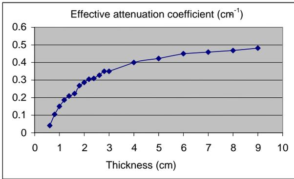
Fig. 2 Effective attenuation coefficient ( $\text{cm}^{-1}$ ) calculated through simulation- configuration A1.
