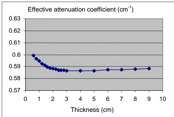
Fig. 4 Effective attenuation coefficient ( $\text{cm}^{-1}$ ) calculated through simulation- configuration A2.
