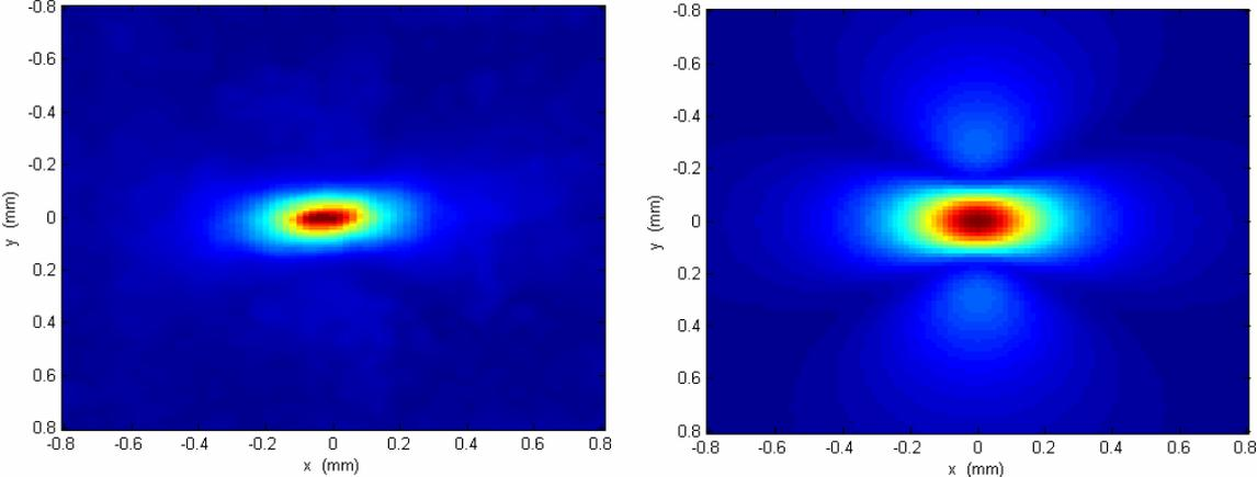
**Fig. 8:** Experimental CSCAN mapping of the  $200 \times 100 \times 200 \mu\text{m}$  flaw (left part), and comparison with the simulated results (right part) in the case of  $B_x$  measurement.
