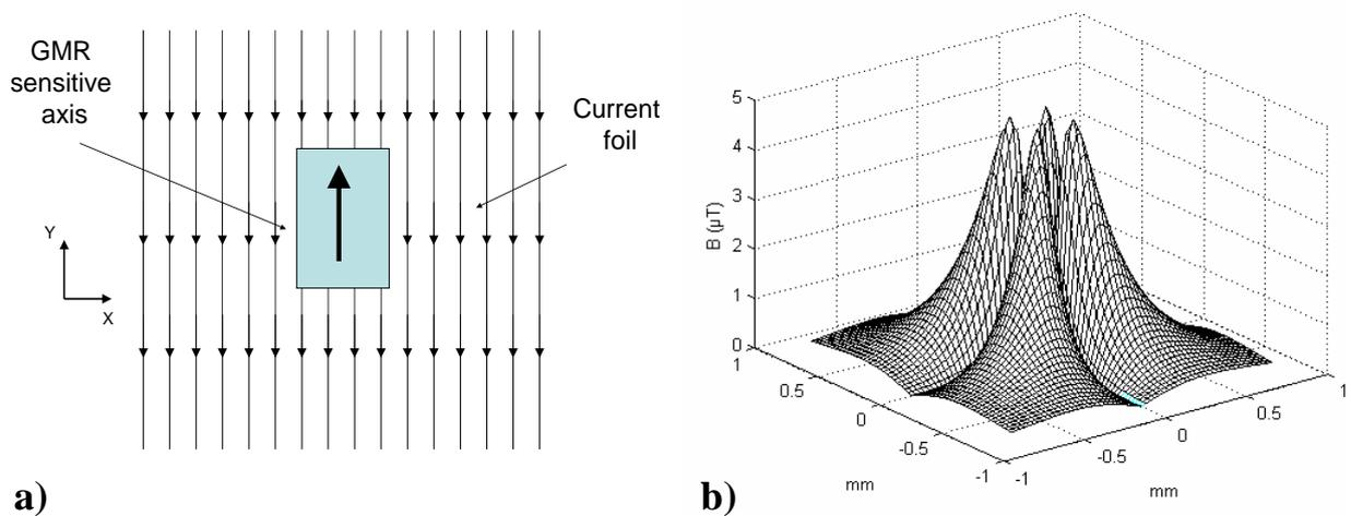
**Fig. 5:** (a) Description of the « $B_y$ » configuration; (b)  $B_y$  component of the magnetic field due to the presence of a surface breaking flaw ( $100*100*100 \mu m$ ).
