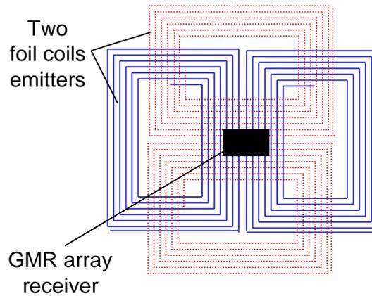
**Fig. 6:** Description of the probe based on a GMR array receiver and two current foils emitters.
