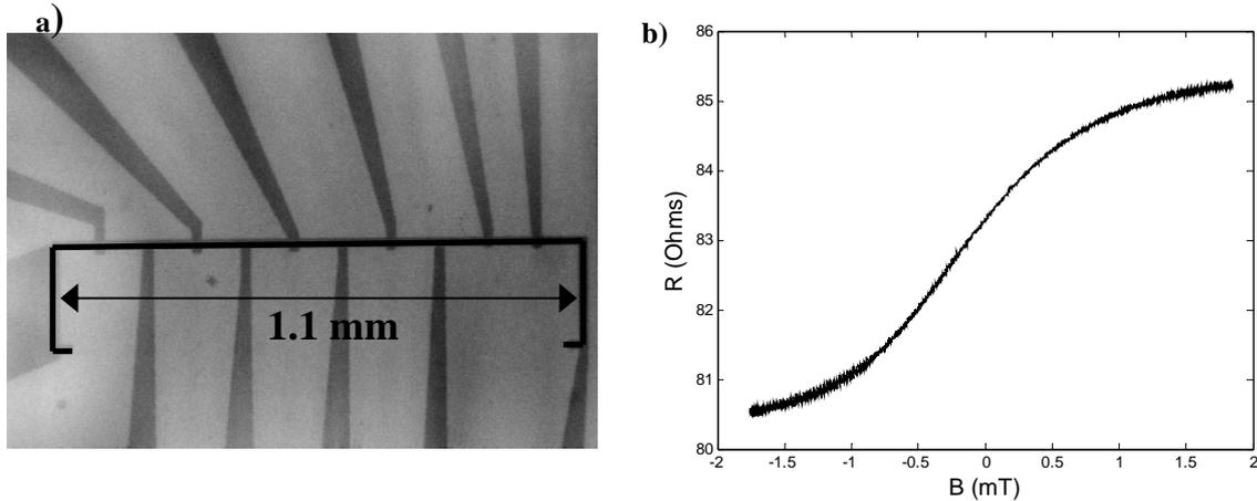
**Fig. 3** Description of the GMR sensor: a) Photo of the GMRs array probe. b) GMR characteristics as a function of the applied field.
