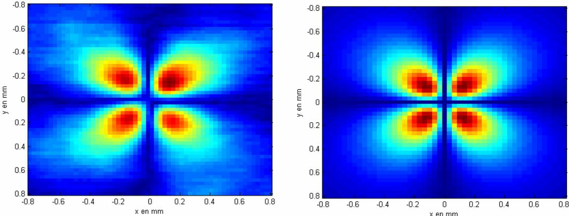
**Fig. 9** Experimental CSCAN mapping of the  $200 \times 100 \times 200 \mu\text{m}$  flaw (left part), and comparison with the simulated results (right part) in the case of  $B_y$  measurement.
