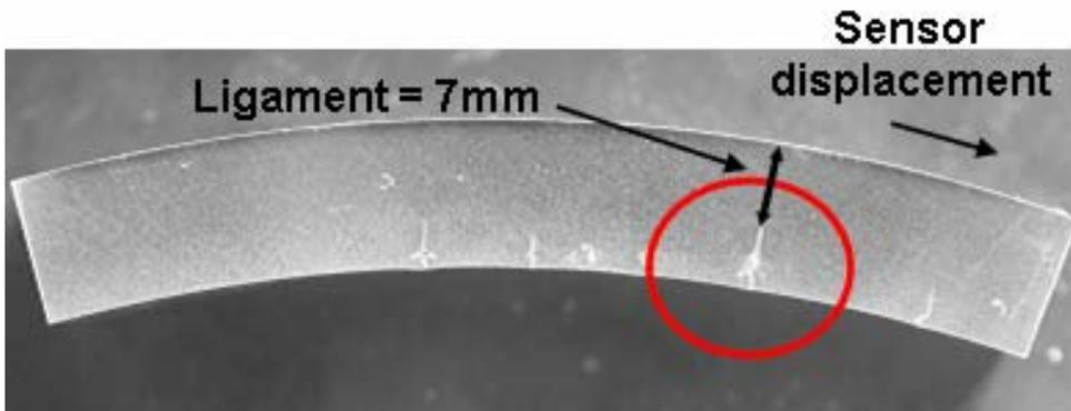
**Fig. 1:** Transverse section of the 316L pipe affected by cracking and crazing induced by thermal fatigue.
