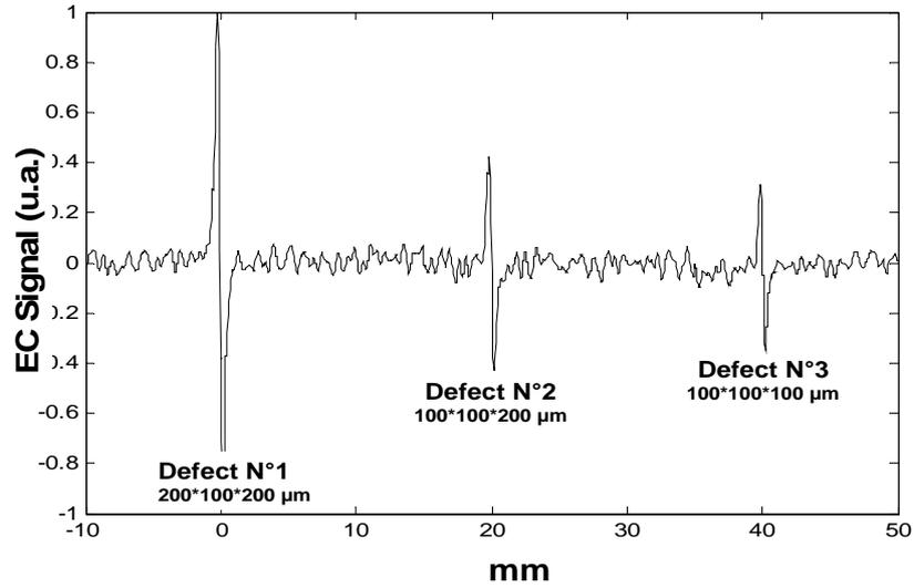
**Fig. 10:** EC signal obtained for the detection of small surface breaking flaws by the GMR probe in the case of the By field measurement.
