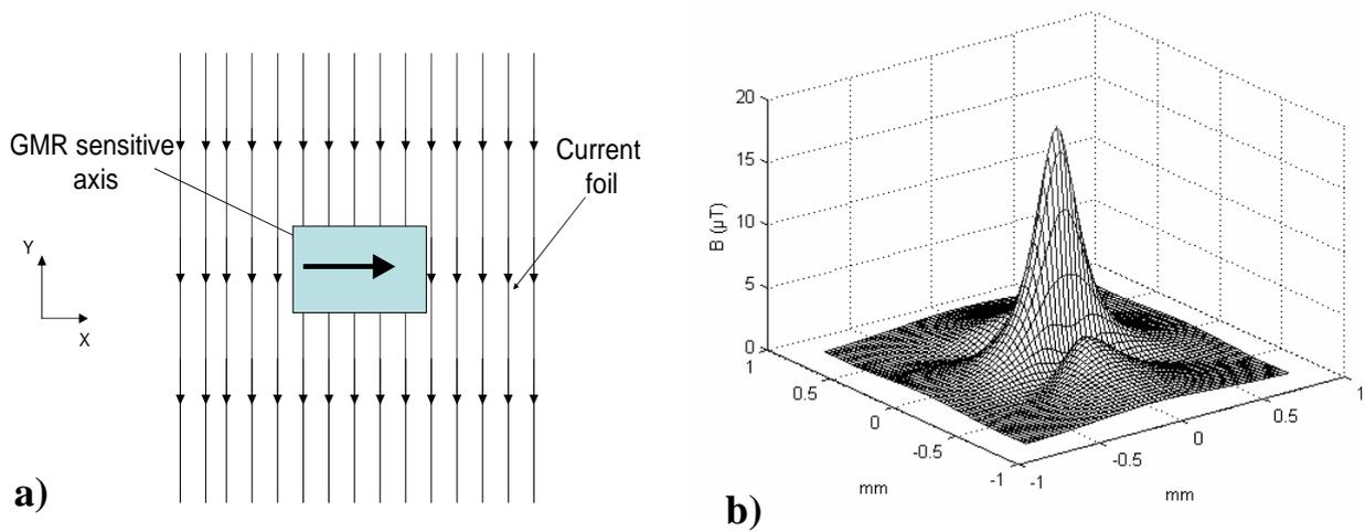
**Fig. 4:** (a) Description of the « $B_x$ » configuration; (b)  $B_x$  component of the magnetic field due to the presence of a surface breaking flaw ( $100*100*100 \mu m$ ).
