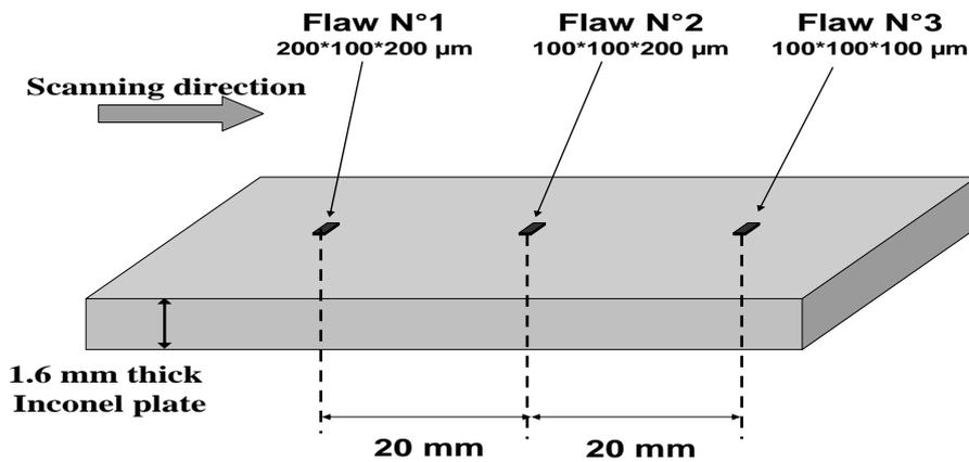
**Fig. 7:** Description of the experimental mock-up.
