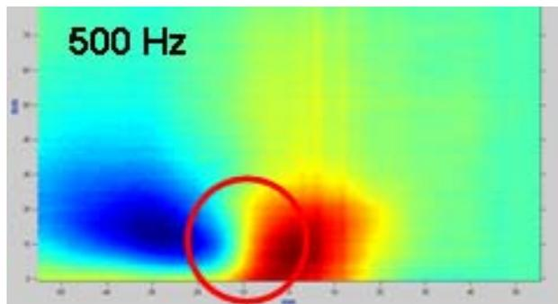
**Fig. 2 :** CSCAN mapping obtained at 500Hz with a GMR receiver for the detection of a deeply embedded flaw under a ligament of 7mm.
