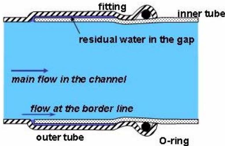
**Fig. 1:** The problem of the assembly of residual water within the gap between the metallic tubes and the fitting structure was investigated in this study under different experimental conditions
