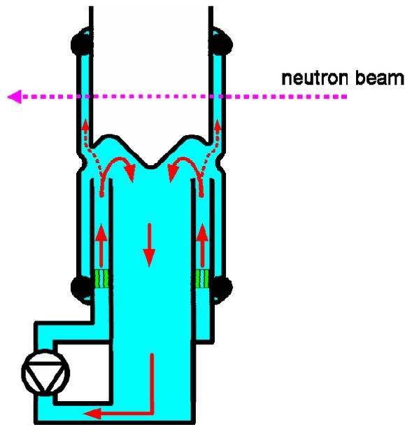
**Fig. 2:** Principle setup for the study of the streaming conditions of water in the gap between tubes and the fitting under different conditions. The real device is shown in Fig. 3.
