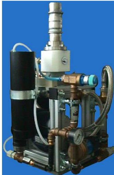
**Fig. 3:** Test facility for the on-site diagnostics of the water flow in the fitting region, based on the scheme in Fig. 2. The dimensions become clear if the tube (on top) diameter of 8 cm is taken into account.
