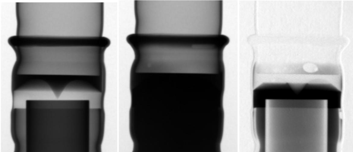
**Fig. 4:** Neutron images of the inspection zone of the setup in Fig. 3: left – the empty assembly, middle – after water filling, right – after “referencing” according to (2)
