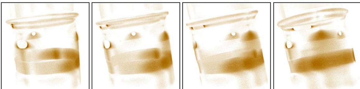
**Fig. 6:** Water distribution inside the metallic structure of the fitting. Even if only thin films remain, the neutron tomography method has sufficient sensitivity to detect the water.
