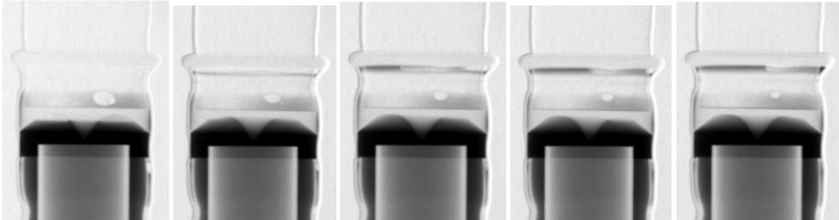
**Fig. 5:** Filling process of the asymmetric steel fitting with normal water in a sequence of images. Obviously, the residual air content plays a role how and where the water can migrate. The first image was taken directly after starting of the pressure application. The final state was reached after about 15 minutes.
