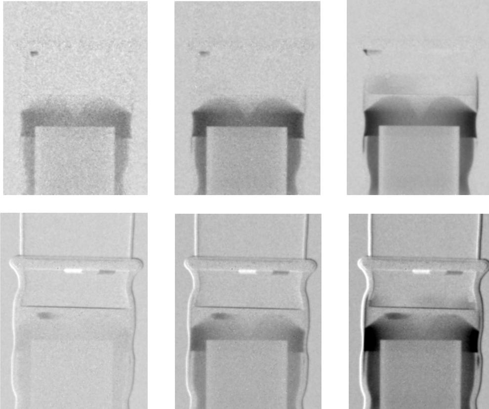
**Fig. 7:** Water exchange during recirculation of light water replacing heavy water, which was used previously in the initial filling: upper line – symmetric structure, lower line – asymmetric structure. The process is followed over a time interval of up to 30 minutes
