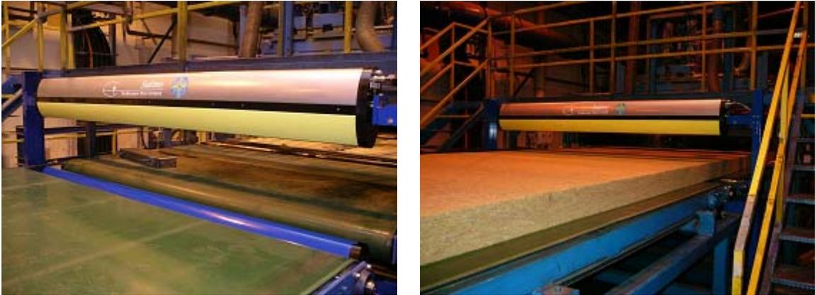
Figure 10 : Non invasive system installed on a stone wool production line
