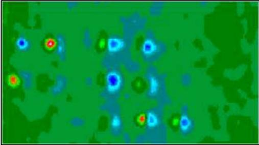
Fig 7 Aluminium Honeycomb with defects
