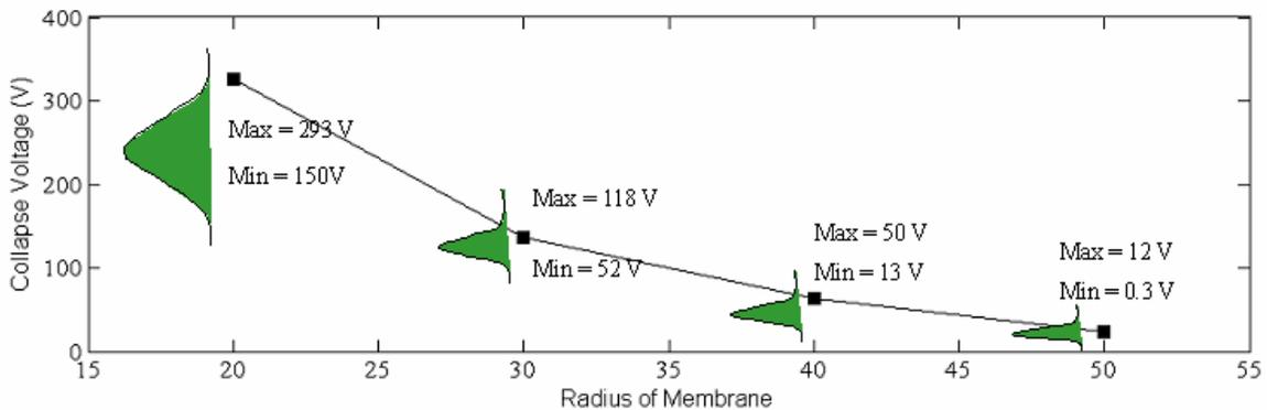
Figure 8: Comparison of Probabilistic Design with deterministic model
