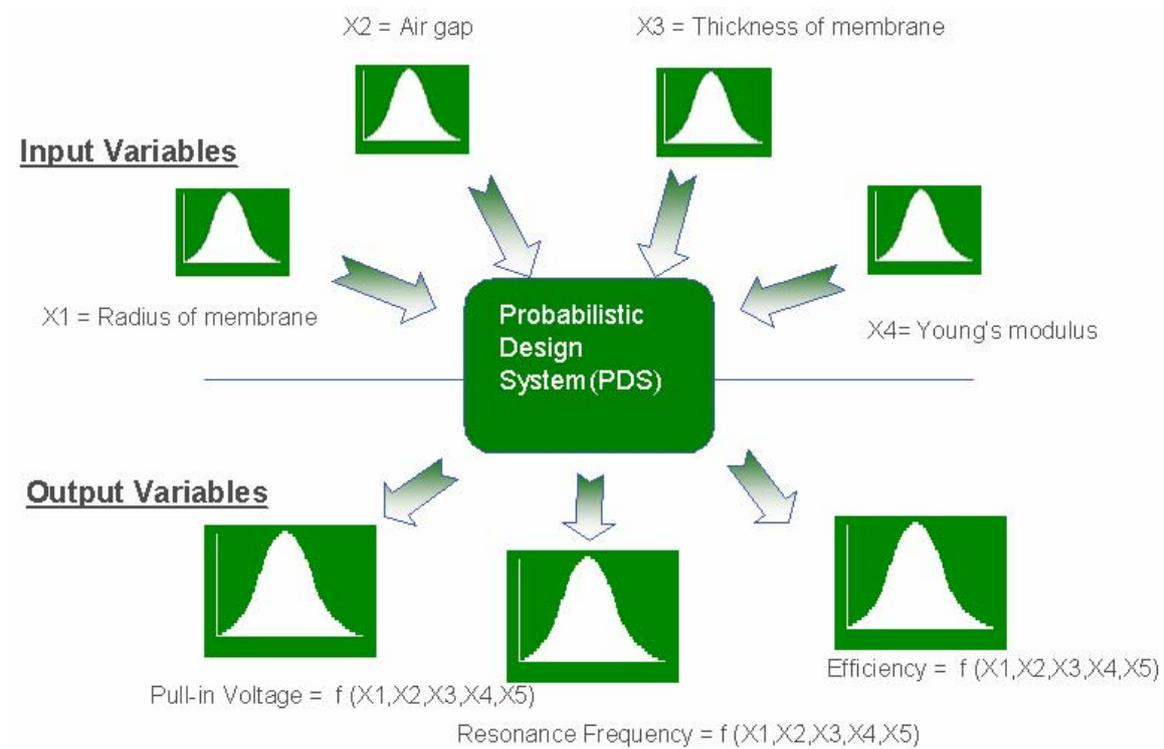
Figure 4: Schematic on the working of PDS
