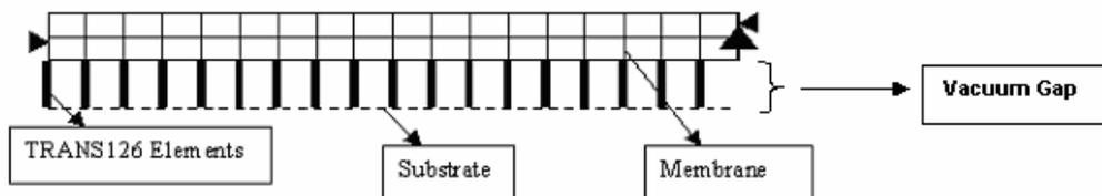
Figure 3: Direct coupled field finite element model
