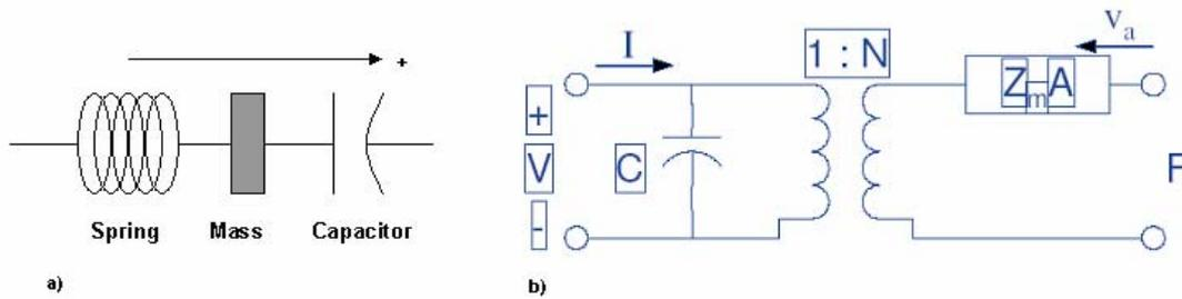
Figure 1: a) Mass spring model b) Equivalent circuit model
