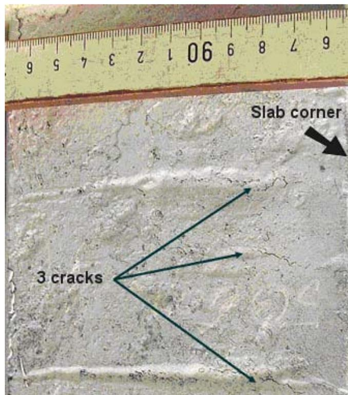
**Figure 12:** result of magnetic particle inspection: the crack detected with the eddy-current array probe was the top one.
