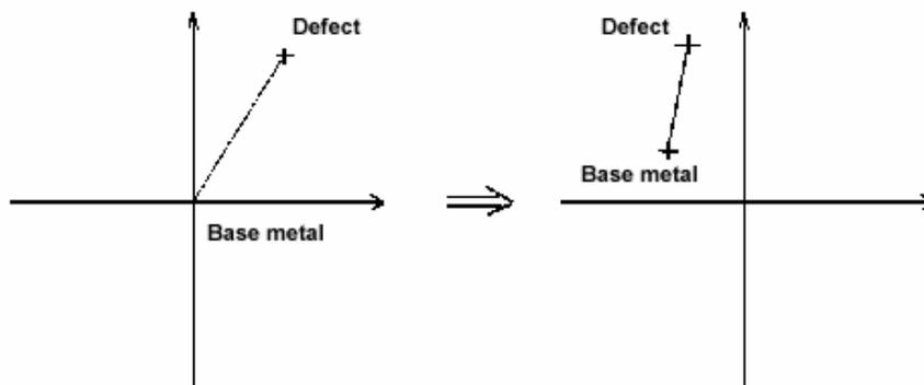
**Figure 3:** Effect of a perturbation on the probe signal in the impedance plane
