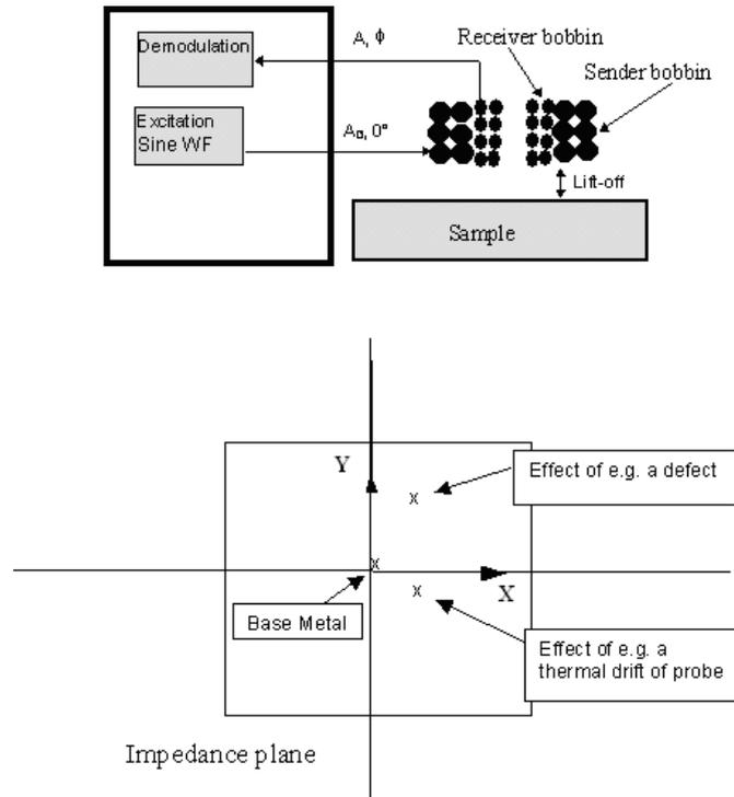
**Figure 2:** Eddy-current inspection schematics and impedance plane representation
