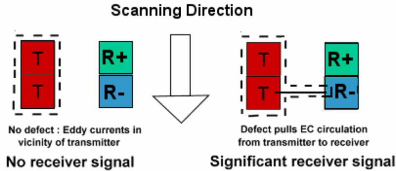
**Figure 5:** Transmit receive principle with 2 transmitter coils and 2 differential receiver coils
