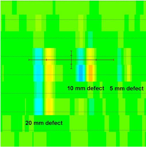
**Figure 8:** Detection of small cracks with a 4.5 mm square element dual line array probe, operating with 3 mm lift-off.
