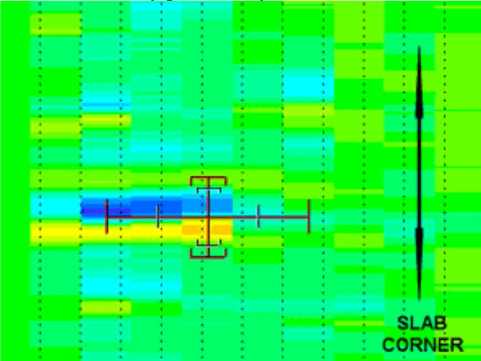
**Figure 10:** Probe response over a rough surface, outlining a crack. The arrow gives the position of the slab corner along the 45 mm wide C-scan. The crack is transverse to the casting direction; probe movement is also along casting direction.
