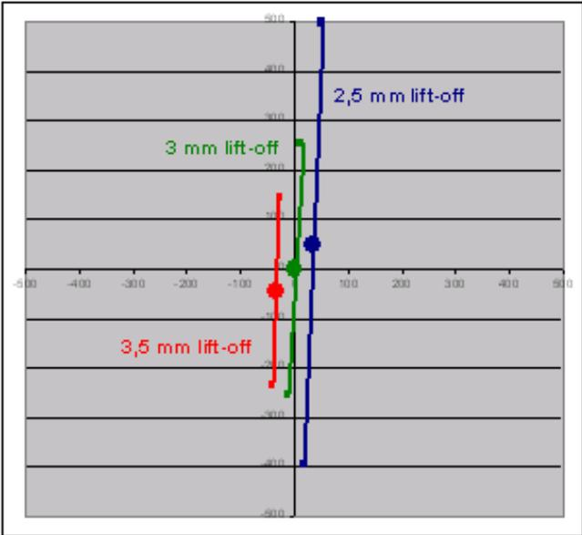
**Figure 9:** Effect of lift-off variations around nominal 3 mm lift-off for the 4.5 mm square element dual line array probe
