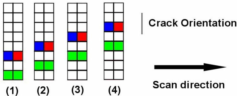
**Figure 6 :** First four time windows for a differential anisotropic eddy-current probe; transmitter elements are in green, differential receivers in blue and in red.
