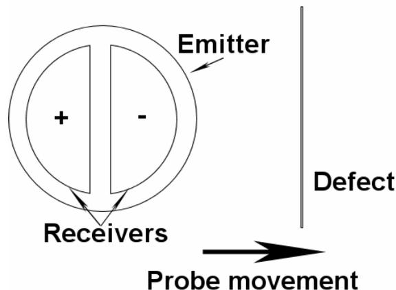
**Figure 4:** Differential Double D type pick-up coil
