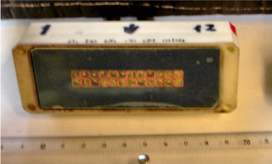
**Figure 7:** 4.5 mm square element dual line array probe.
