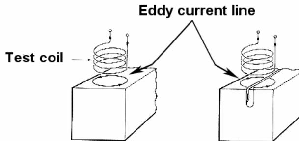
**Figure 1:** A surface crack will modify the surface current distribution
