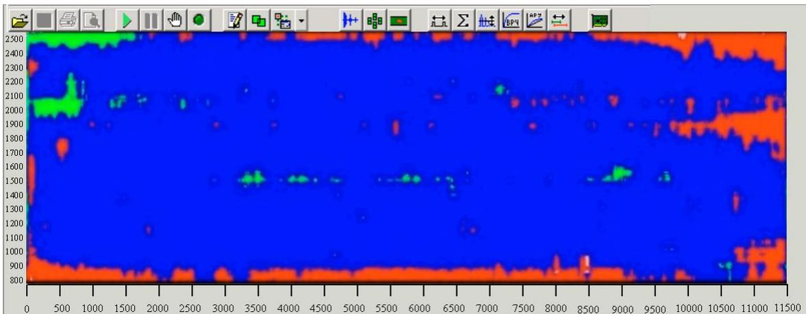
**Figure 6.** C-scan of a steel plate indicating areas with abnormal mechanical properties (red and green areas)
