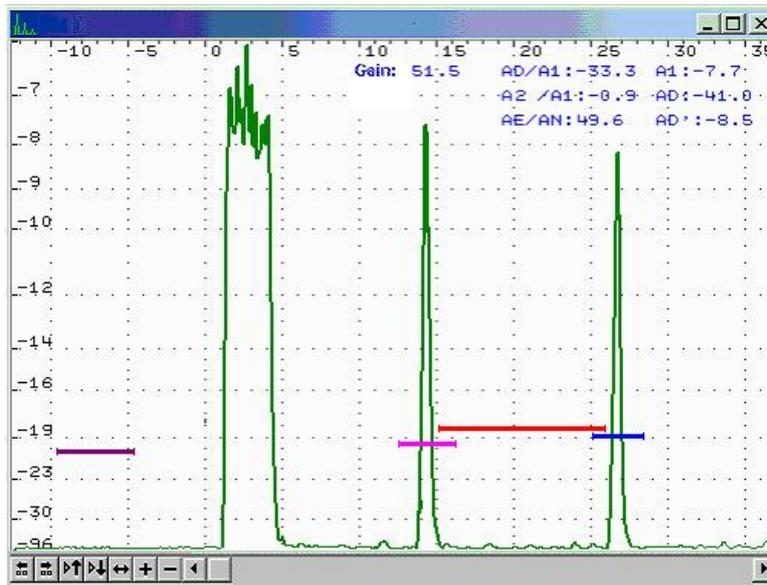
**Figure 1.** A-scan of a defect free area of a 20 mm plate
