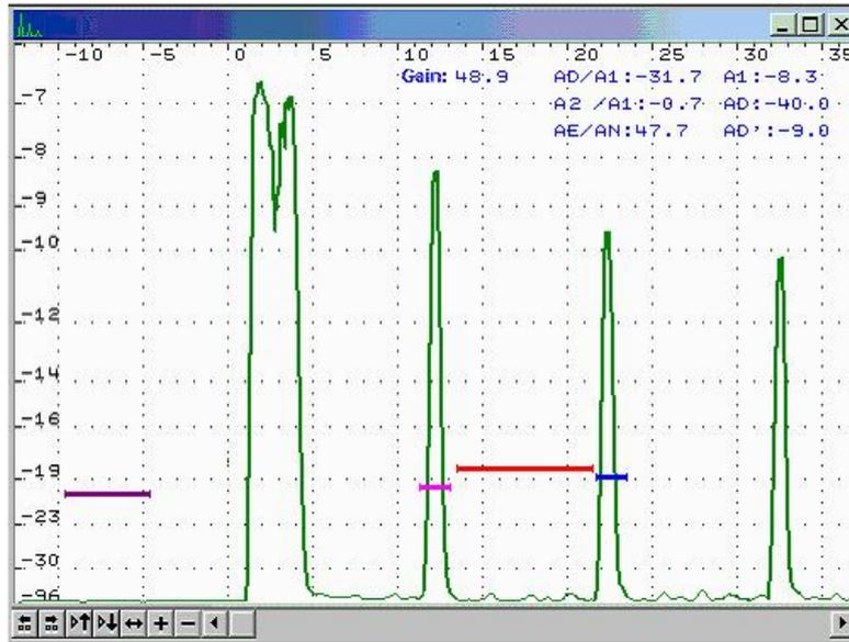
**Figure 3.** A-scan of a defect free area of a 16 mm plate
