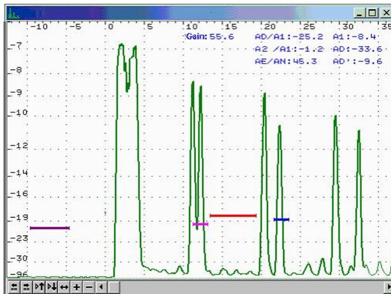
**Figure 5.** A-scan obtained with an EMAT turned by  $45^\circ$  relative to the rolling direction on a defect-free area of a 16 mm plate.
