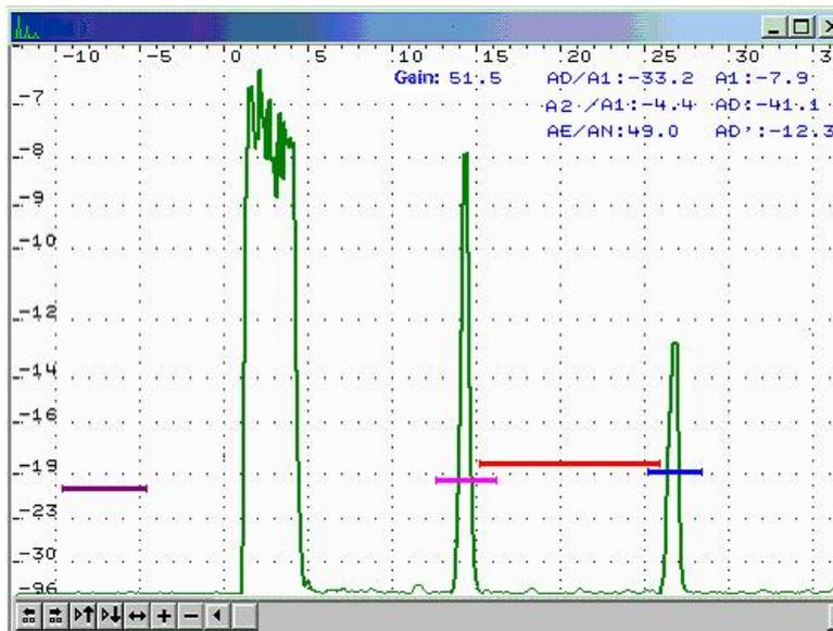
**Figure 2.** A-scan with an artificial scratch 0.3 mm deep in the same 20 mm plate
