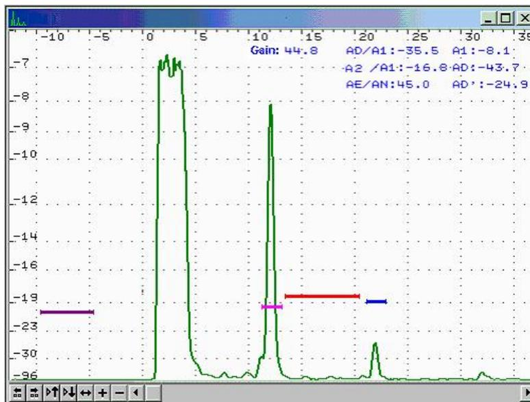
**Figure4.** A-scan with from the area with a natural vertical surface crack in the same 16mm plate
