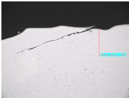
Fig. 12: Metallographic cross section along the arrow direction in Fig. 11a. The crack depth is 0.2 mm
