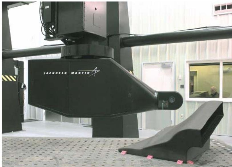
**Figure 3.** LaserUT system inspecting a complex-contoured composite part.
