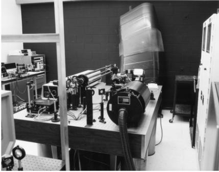
**Figure 1.** Late 80's lab prototype at GD for concept demonstration of inspection of composites.
