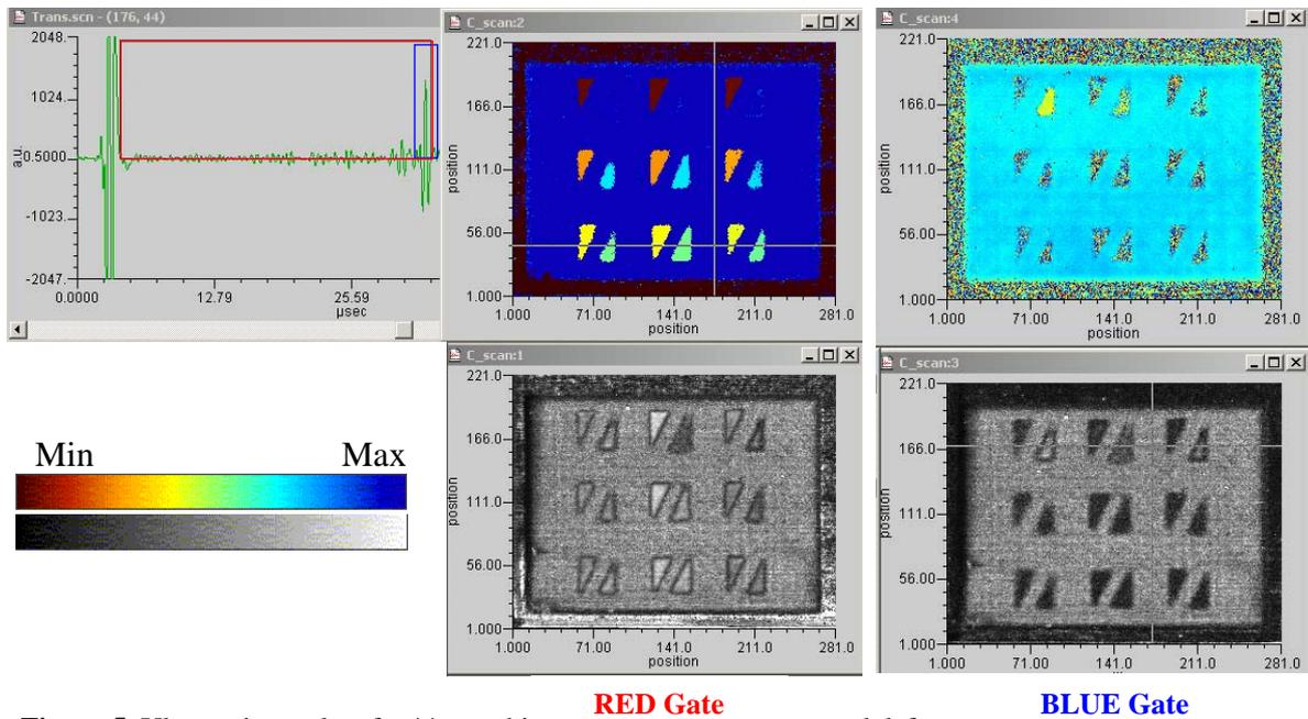
**Figure 5.** Ultrasonic results of a 44 mm thick CFRP block with inserted defects with the LaserUT system. Time of Flight C-scan (Top) and Amplitude C-scan (Bottom).
