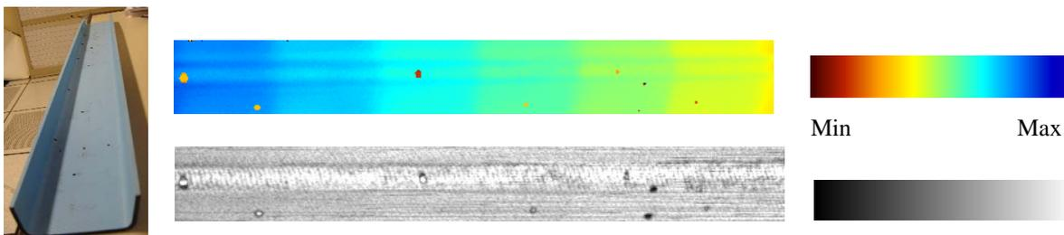
**Figure 6.** Ultrasonic results of a CFRP spar with flat bottom holes ( $\varnothing 2 - 3 - 4$  mm) with the LUIS. Time of Flight C-scan (Top) and Amplitude C-scan (Bottom).
