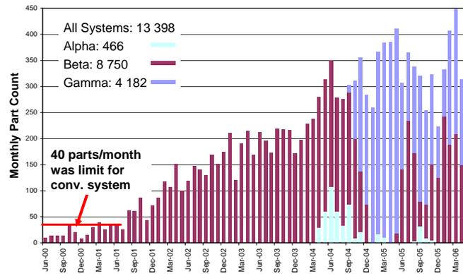
**Figure 4.** Number of parts by month inspected by LaserUT systems at Lockheed Martin Aeronautics at the Fort Worth, Texas facility since the technology was introduced in production in June 2000 as of May 1<sup>st</sup> 2006.
