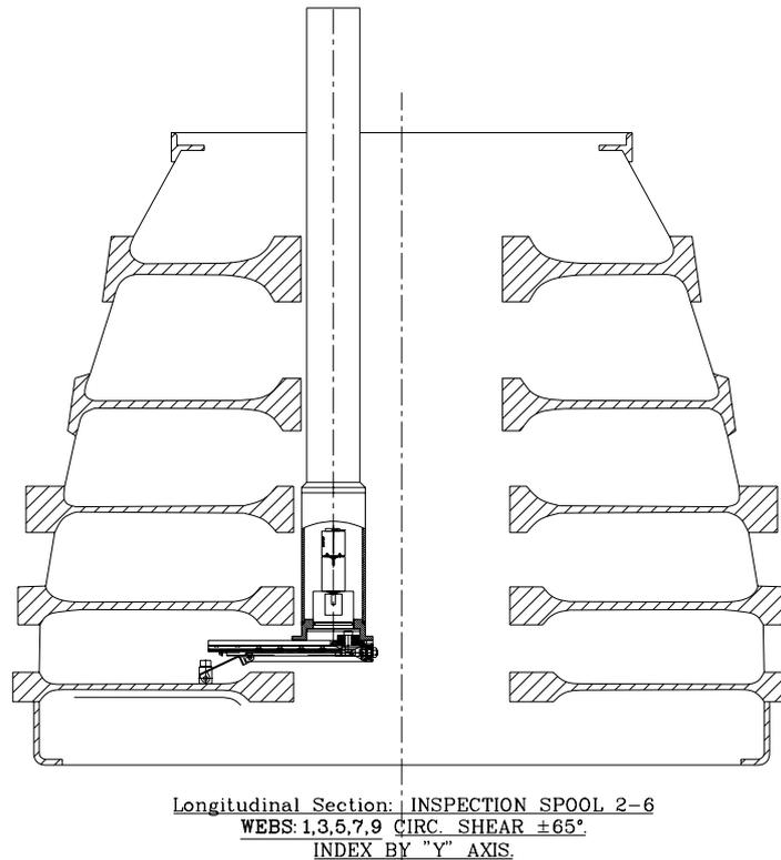
**Figure 6:** Yoke with telescopic device retracted
