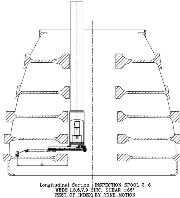
**Figure 5:** Yoke with telescopic device extended
