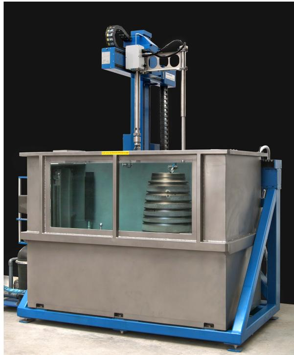
**Figure 4:** Immersion tank
