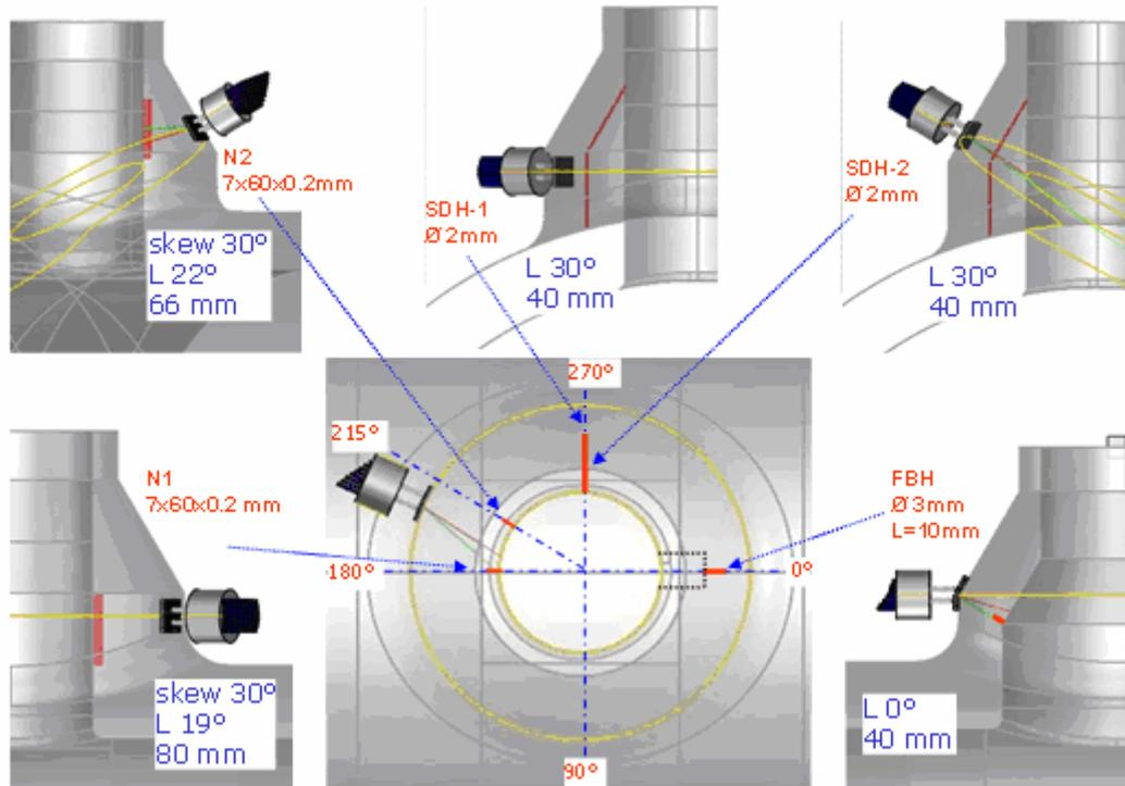
Figure 2: Mock-up summarizing the positions of the defects and the array. Angular positions of the flaws are shown on the central view and details are schematized on lateral views.
