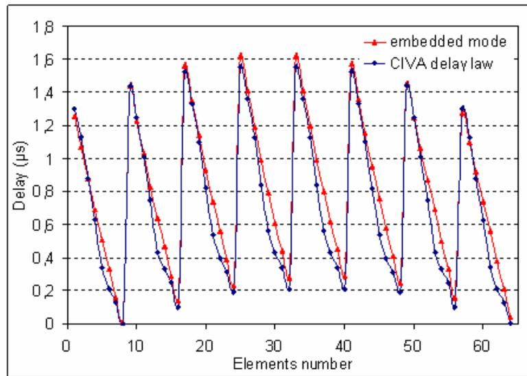
Figure 4 : Delay laws calculated by CIVA on the nominal profile and by the embedded algorithm.
