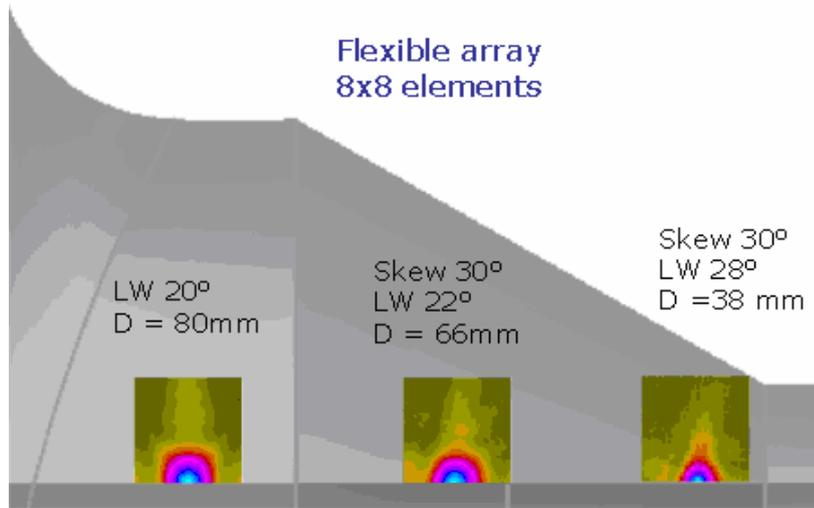
Figure 3: Field calculations with the flexible phased array.
