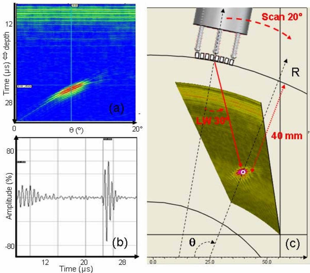
Figure 6 : detection of SDH-2 : presentation of the raw Bscan (a), Ascan (b) and the reconstructed in 3D CAD mock-up
