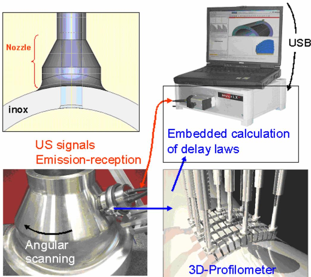
Figure 1: 3-D flexible 8x8 elements array and the acquisition system MultiX 128 parallel channels
