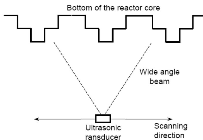
**Fig. 3.** Possible orientation of wide-angle ultrasonic transducer and scanning directions for imaging of the bottom of the fuel channels
