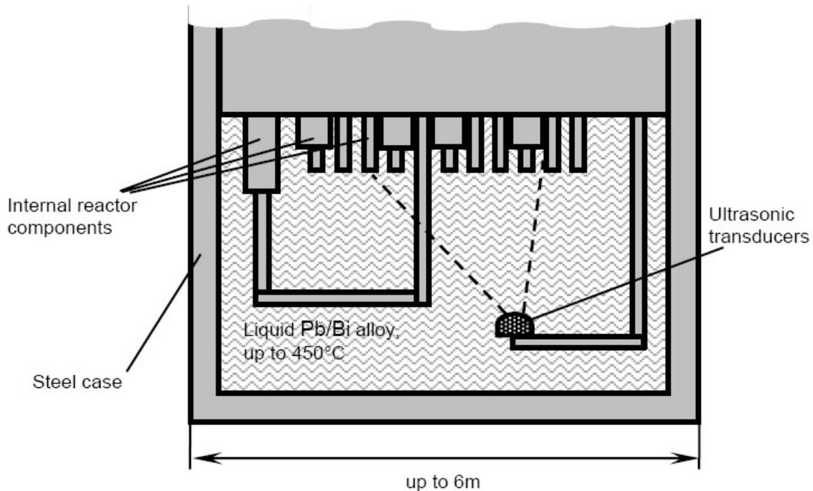
**Fig. 1.** Approximate geometry of MYRRHA reactor
