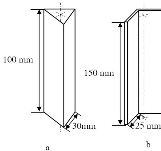
**Fig. 4.** The geometry of the investigated objects: a - triangle prism, b- L-shape profile
