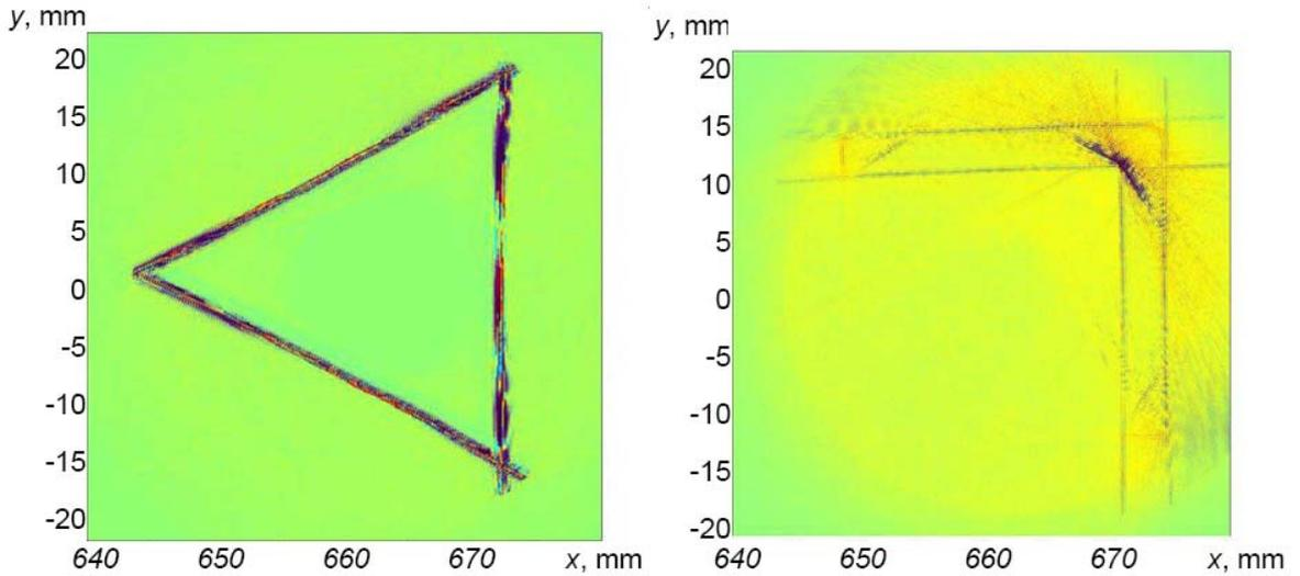
**Fig. 7.** The reconstructed image obtained from the data with the 30dB gain a - of the triangle prism; b - of the L-shape profile
