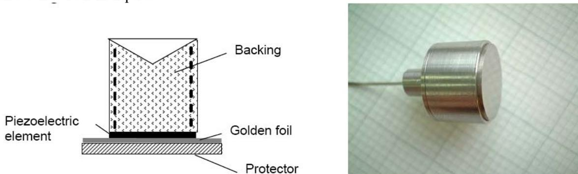
**Fig.2.** a - Sensor with backing and a thin metallic membrane;
