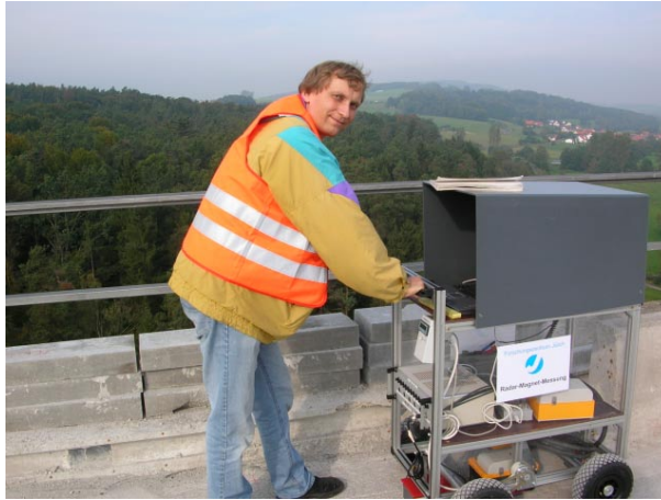
Fig. 9. Radar-Magnetic measurement on the Döllbachtal bridge.
