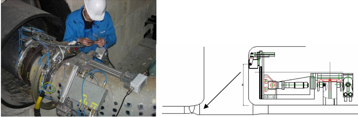
Figure 2: examination of the containment penetration welds
