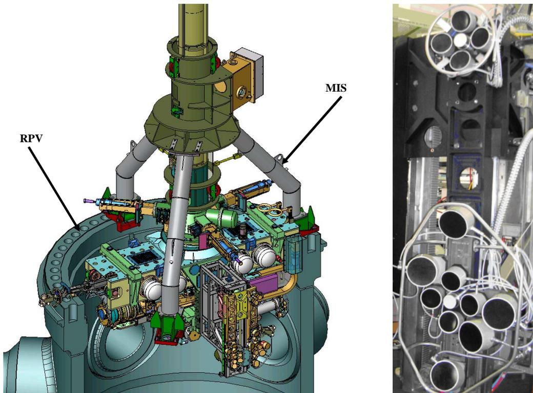
Figure 3: examination of the pressure vessel (manipulator and multi-tool)
