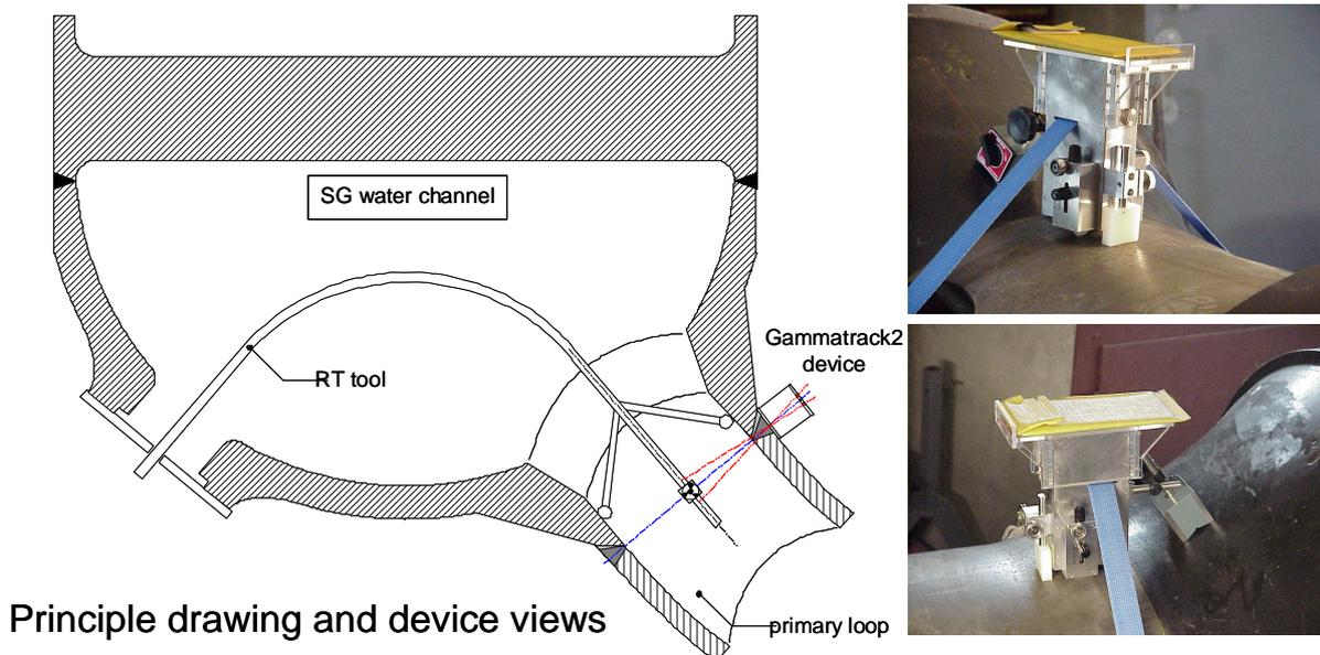
Figure 4: examination of the bimetallic weld between steam generator and primary pipes (GAMMATRACK2 device)
