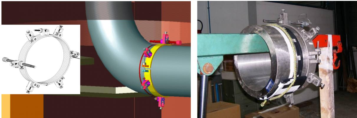
Figure 5: examination of the weld between pipe and elbow of the surge line
