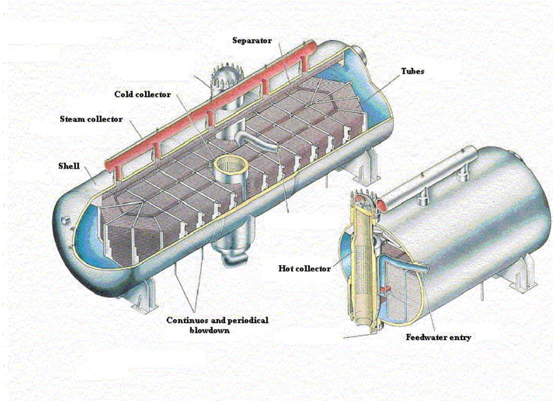
**Figure 4.** Steam generator and heat exchanger tube system
