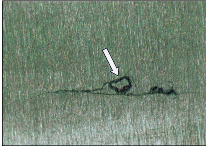
**Figure 5.** A typical defect on the tube outer surface (length of crack is 2.2 mm)
