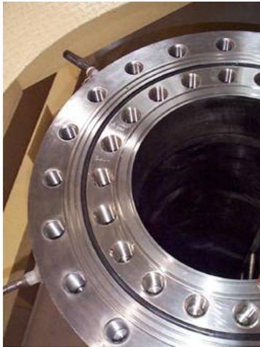
**Figure 2.** Top view of SG primary and secondary collector flanges
