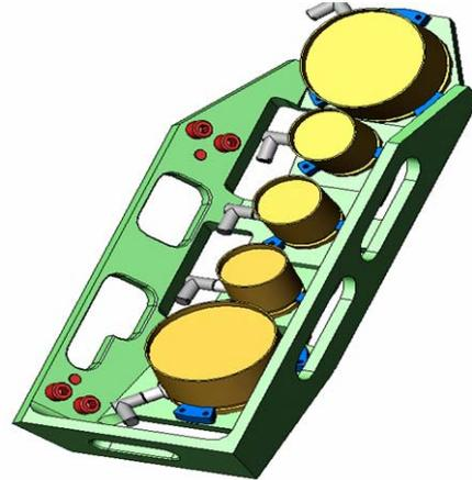
Figure 11 - CAD view of transducers arrangement for nozzle inspection
