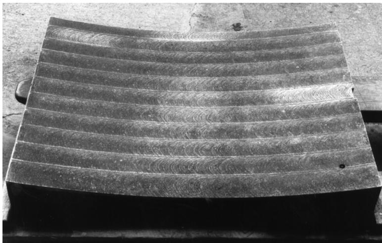
Fig. 3 : Full scale mock-up for the qualification of the UT examination procedure of the core area
