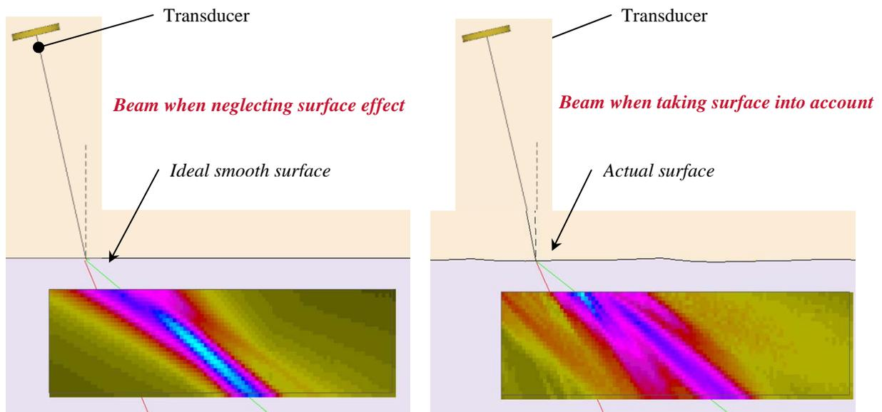
Figure 9 - Computerized UT simulation
