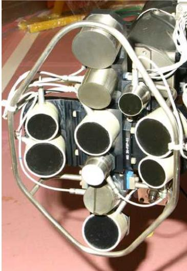
Figure 10 - Transducers arrangement for vessel bottom inspection
