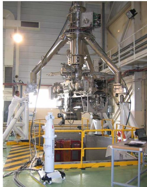
Figure 4 - Checking MIS7 with laser tracker
