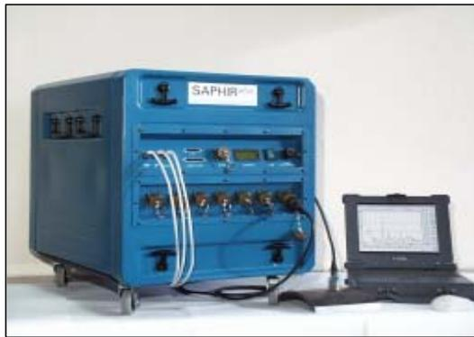
Figure 7 - Saphir<sup>PLUS</sup> phased array UT acquisition system
