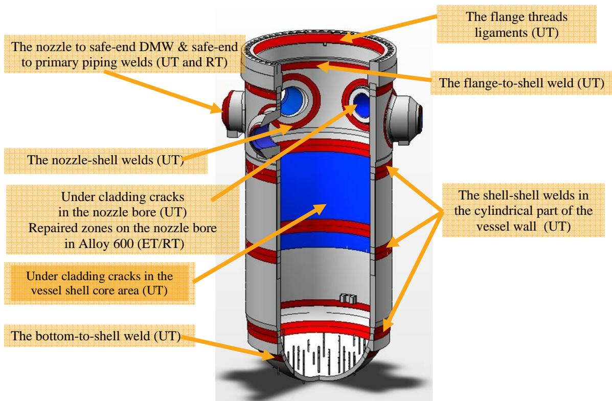
Figure 2 - Target area for RSEM inspection
