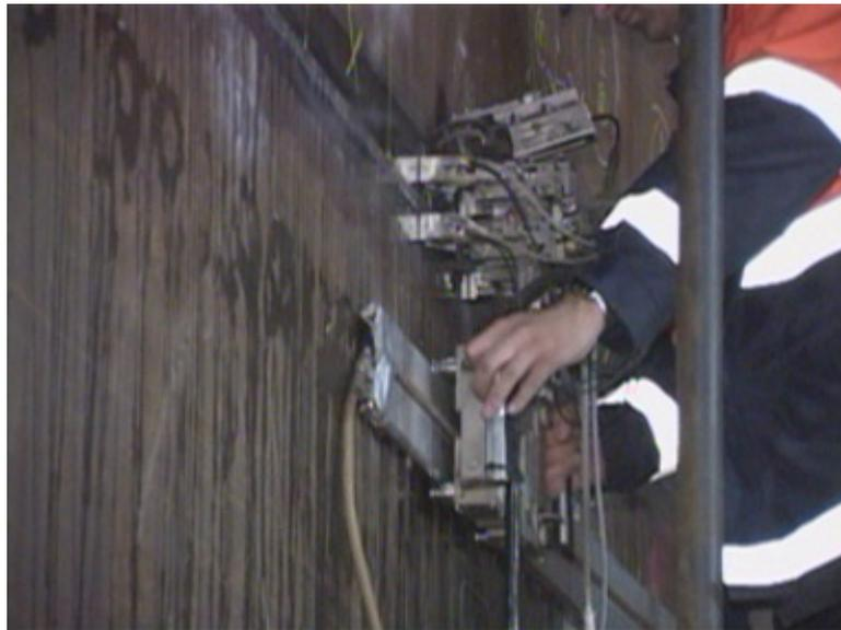
**Figure 3.** Scanning of a 9% Ni LNG storage tank
