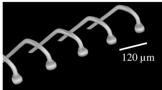
Fig. 2. 3D rendition of Au bonding wires of an IC encapsulated in a glob top against mechanical stresses. Voxel size is 1.6  $\mu\text{m}$ , x-ray energy range approx. 40 to 60 keV.
