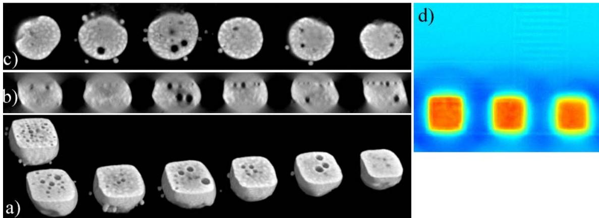
Fig. 3. SRCL inspection of a flip-chip bonded device: 3D rendition of some bump bonds at a device corner (a), two mutually perpendicular slices, perpendicular (b) and parallel (c) to the device surface. The coloured image (d) features a detail of metallisation layers on the hidden surface of the IC. Voxel size is 1.6  $\mu\text{m}$ , x-ray energy range approx. 40 to 60 keV.
