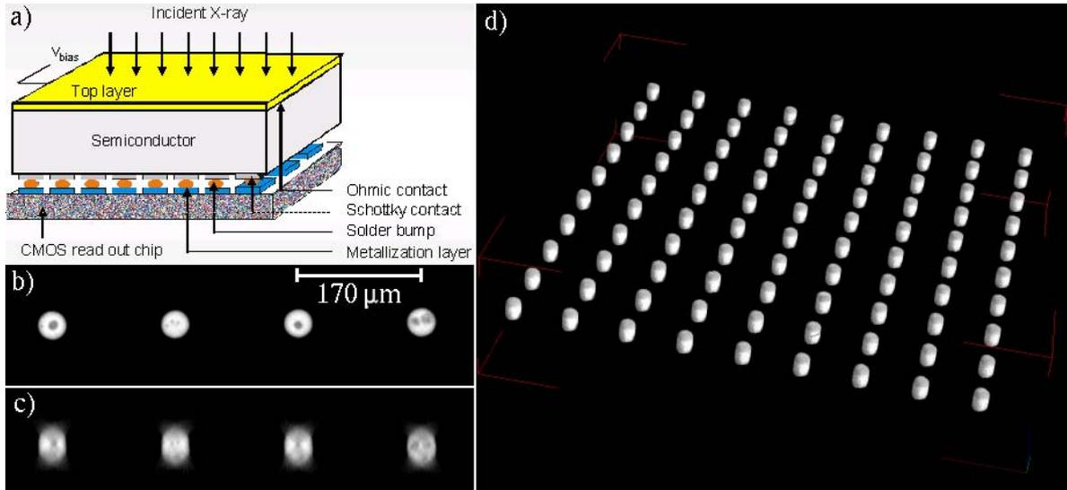
Fig. 4. SRCL inspection of a hybrid detector array with a GaAs semiconductor sensor layer: sketch of the device (a), two mutually perpendicular slices, parallel (b) and perpendicular (c) to the device surface, and a 3D rendition (d) of the centre of the 2d array of bump bonds. Voxel size is 1.6  $\mu\text{m}$ , x-ray energy range approx. 40 to 60 keV.
