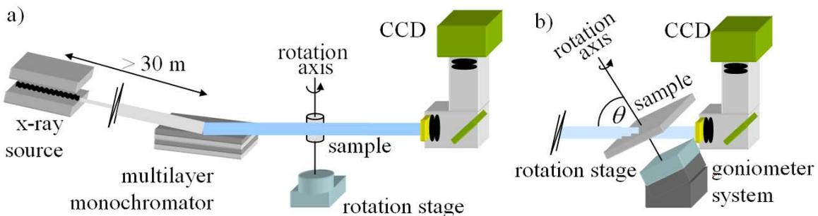
Figure 1: Comparison between the experimental set-ups for computed tomography (a) and computed laminography (b), as implemented at beamline ID19 of the ESRF.
