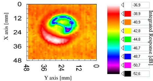
**Figure 16.** Detail of the acquisition with Delta Technique on the CFRP panel; the map reports the Integrated Response ( $\delta = 6$  dB).
