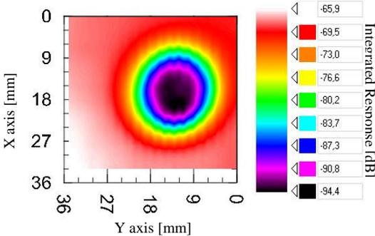
Figure 17. Detail of the transmission inspection on CFRP panel ( $\delta= 18$  dB).
