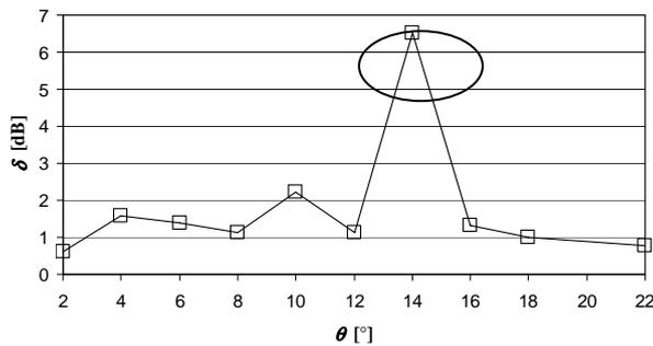
**Figure 13.** Parametric study in function of relative angle between the transducers in Delta configuration;  $b=60\text{ mm}$ ,  $h=90\text{ mm}$ .
