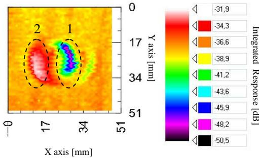
**Figure 15.** Detail of the acquisition with Pitch&Catch technique on the CFRP panel; the map reports the Integrated Response ( $\delta = 7$  dB).
