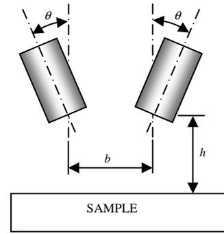
**Figure 12.** Direct Pitch&Catch transducers setup parameters
