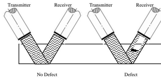
**Figure 2** – Scheme of *direct* Pitch&Catch technique (signal amplitude is attenuated).
