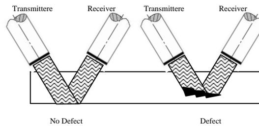
**Figure 3** – Scheme of *indirect* Pitch&Catch technique (time of flight is reduced and the signal amplitude can be enhanced).
