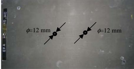
**Figure 9.** Honeycomb sample, with the defects localization .
