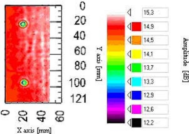
Figure 18. Attenuation map measured on the honeycomb panel using electro-capacitive probes in Pitch&Catch ( $\delta= 3$  dB).
