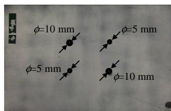
**Figure 8.** CFRP sample, with the defects localization.
