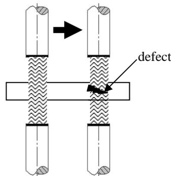
**Figure 1.** Inspection through transmission configuration for non contact ultrasonic technique.
