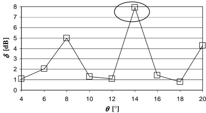
**Figure 11.** Parametric study in function of relative angle between the probe in direct Pitch&Catch and the normal to the inspected plane;  $b=60\text{mm}$ ,  $h=90\text{ mm}$ .
