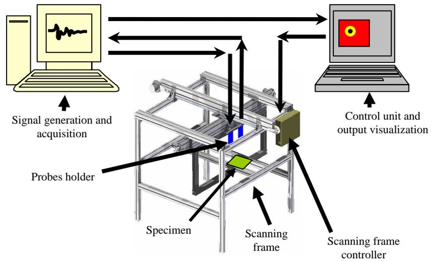
**Figure 5.** Sketch of the test bench main components.
