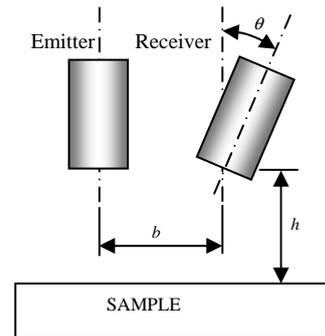
**Figure 14.** Delta transducer setup parameters.
