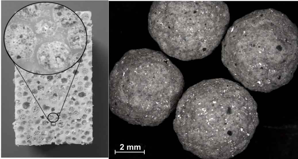
**Figure 1.** Syntactic foam with a polymer matrix (left) and ceramic grains (right) [1].
