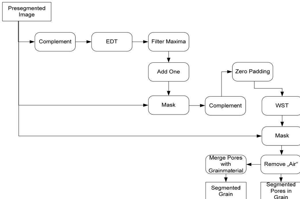
**Figure 6.** Processing chain for segmentation of the ceramic grain and its individual pores (EDT: Euclidean Distance Transformation, WST: Watershed Transformation).
