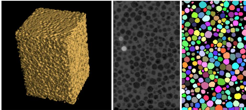
**Figure 3.** Syntactic foam – polymer matrix with KeraPlus grains.
