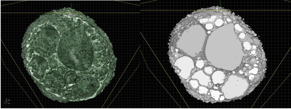
**Figure 7.** Volume rendering of a ceramic grain (left) and the segmented pores (right).
