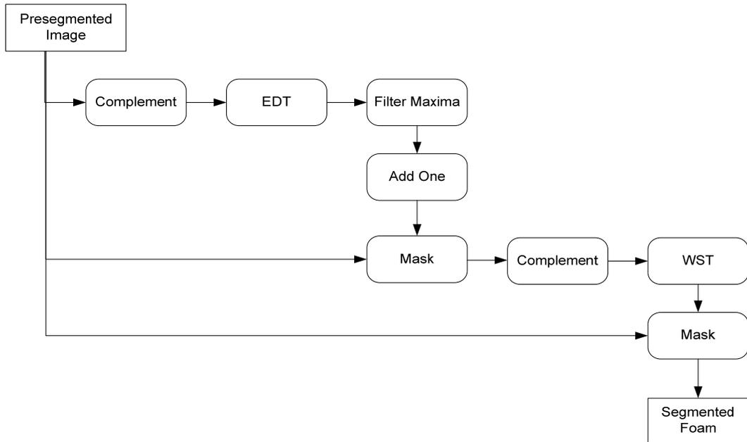
**Figure 2.** Processing chain for segmentation of the grains in the syntactic foam (EDT: Euclidean Distance Transformation, WST: Watershed Transformation).
