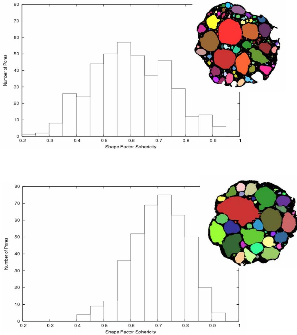
**Figure 8.** Histograms of the shape factor sphericity of pores. Above KeraPlus4–8a for pores with diameter larger than 0.25mm and below 0.174mm for KeraBims4–6a, respectively. Lower bounds chosen according to the respective volumes of 142mm<sup>3</sup> and 48mm<sup>3</sup>. (Visualisation of slices through the segmented pore structure in the respective upper right corners.)
