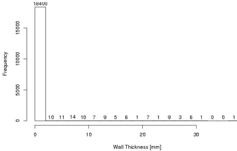
**Figure 4.** Histogram of the grain-to-grain distances in the syntactic polymer foam. The resolution was 0.24mm.
