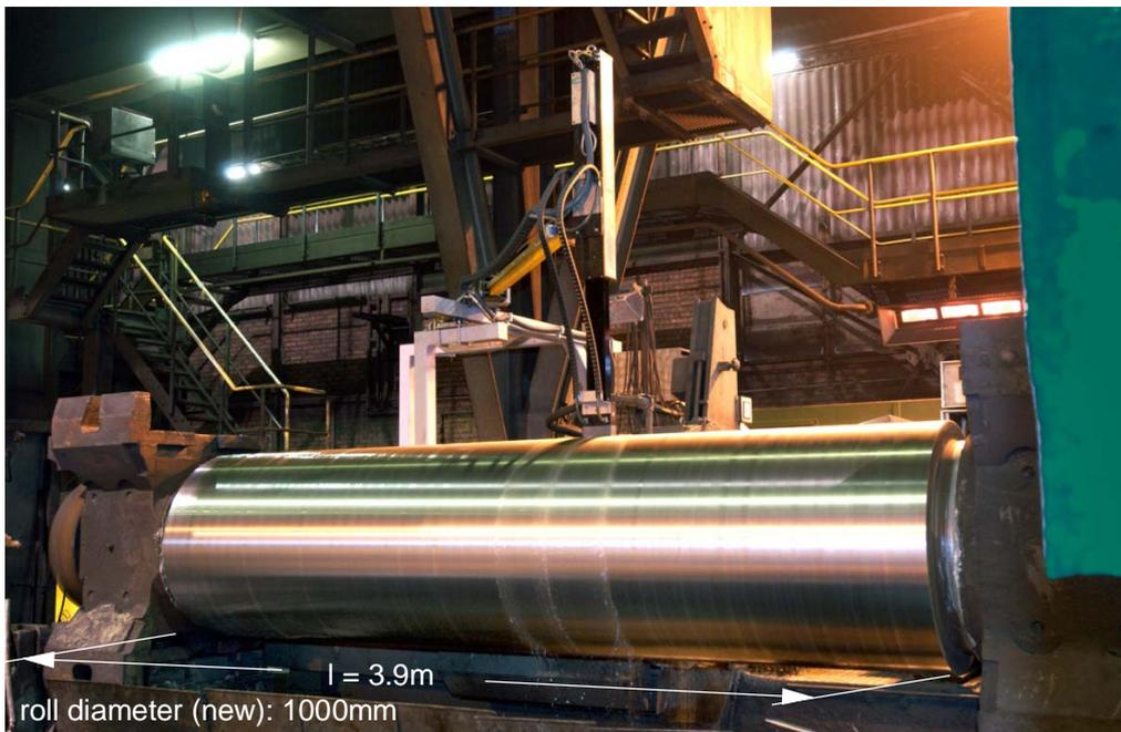
Figure 2: General view of the testing system in the mill shop of the heavy plate profit centre (PCG) of ThyssenKrupp Steel AG
