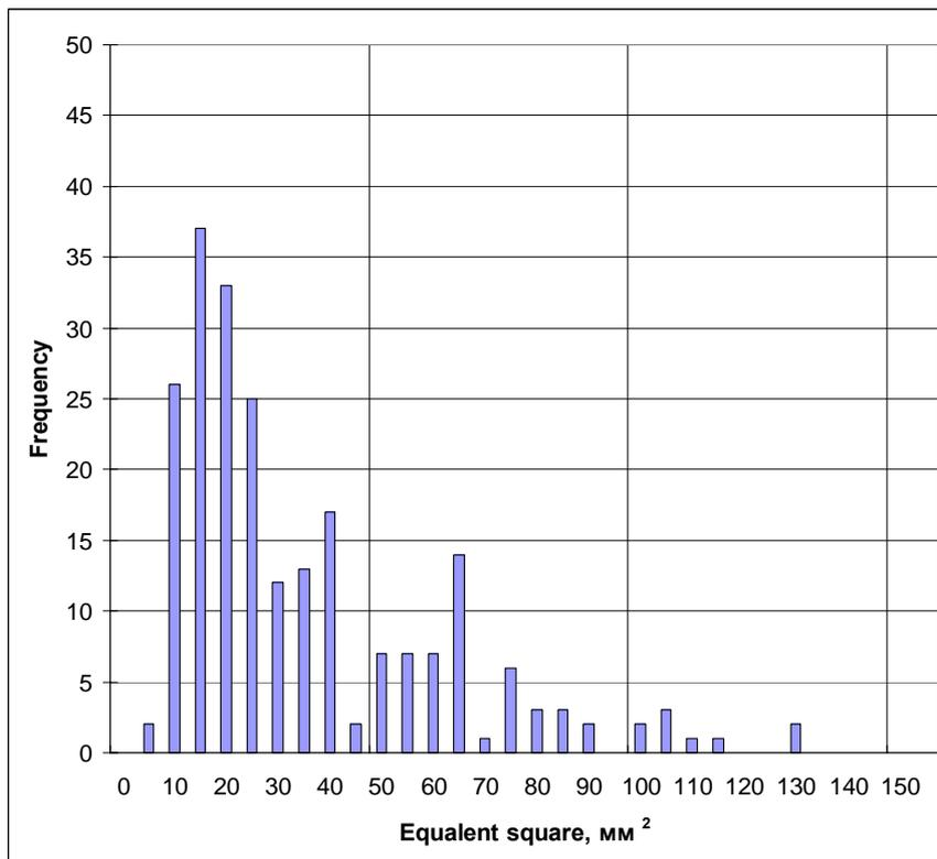
**Figure 2.** Distribution of flaws in backup roll by sizes.
