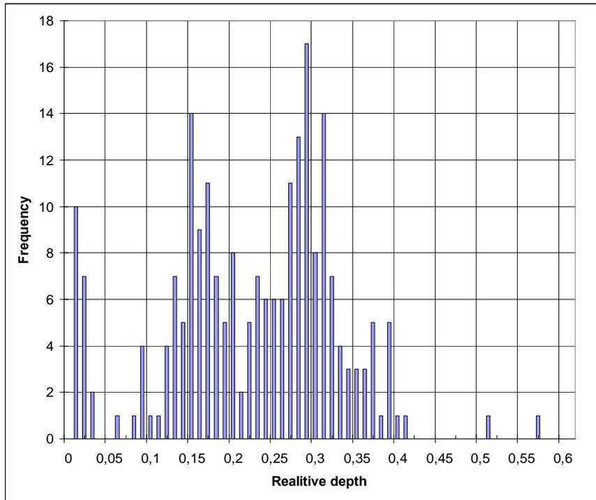
**Figure 1.** Distribution of flaws in backup roll mill.
