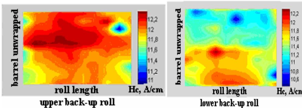
Fig. 6. Inhomogeneous distribution of stress in a couple of backup rolls, caused by out-of-roundness of one of them [3]
