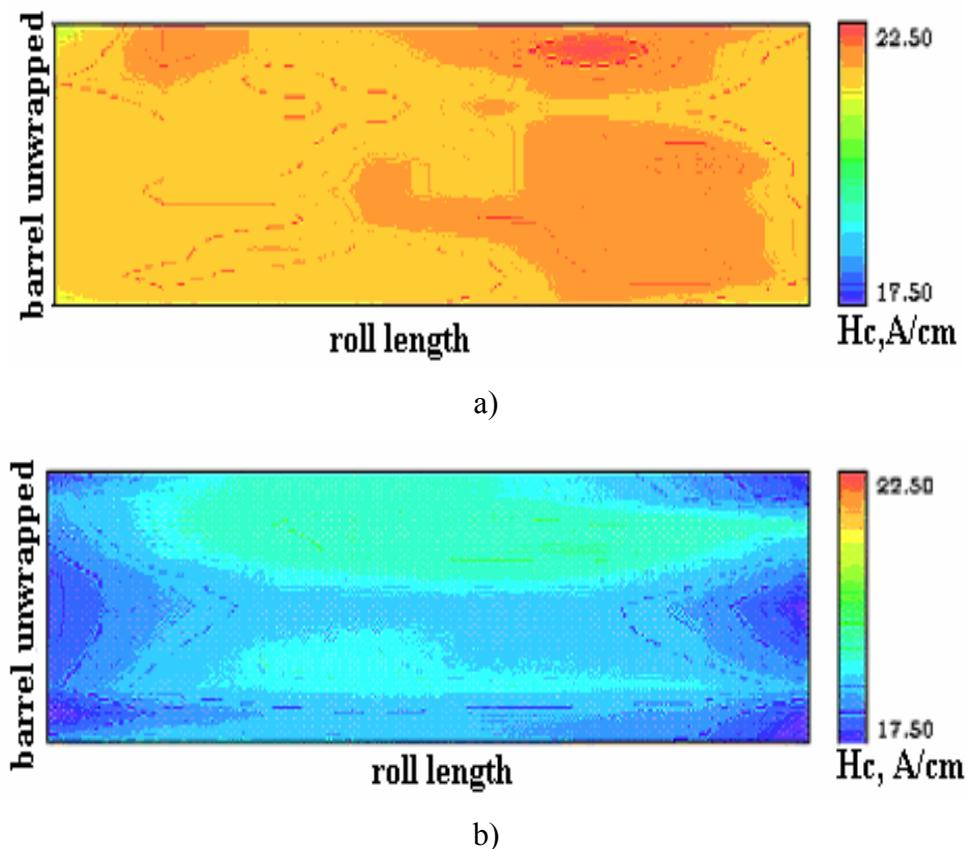
Fig.2. Magnetic chart of iron working rolls produced by different suppliers
