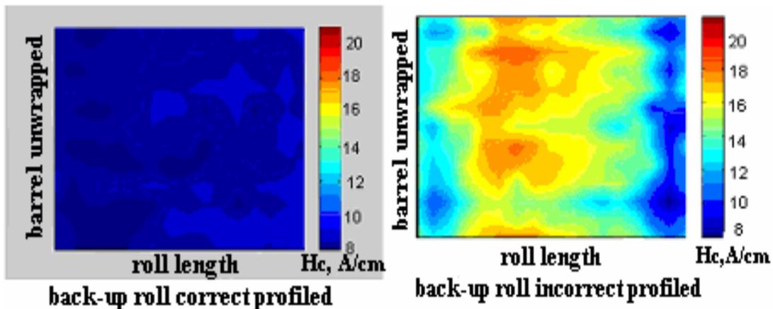
Fig.8 Two similar backup rolls after approximately 40,000 tonnes of cold rolled sheet [8]
