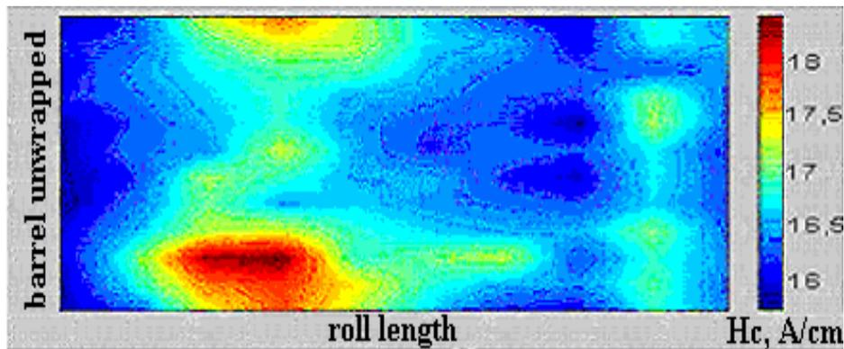
Fig.3. The damage trace in the working layer of the roll barrel.
