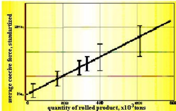
Fig.5. Alignment chart for calculation of residual resource of a cold rolling mill backup rolls [3]
