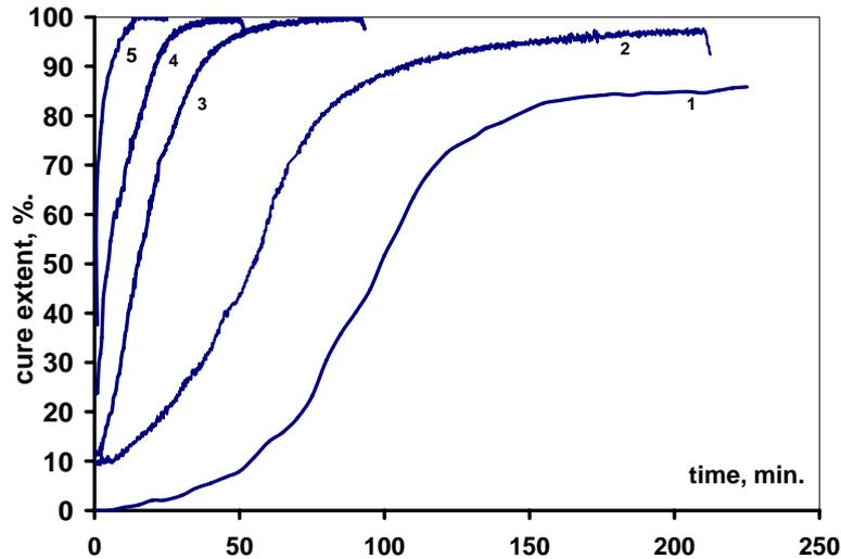
Figure 3. Acoustic extent of the cure reaction. Notes are the same as in Fig. 1.
