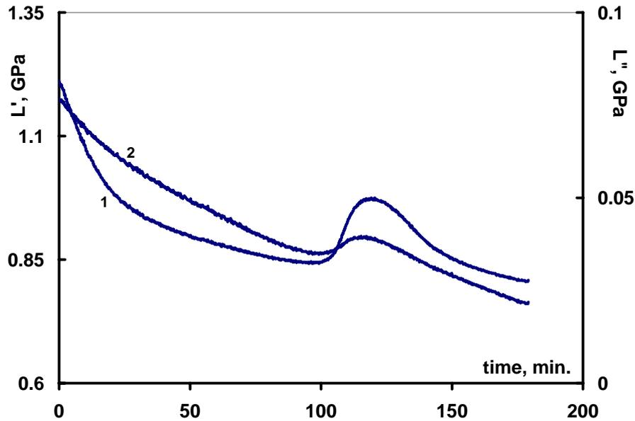
Figure 5. Changes in adhesive loss  $L''$  (1) and storage  $L'$  (2) moduli during non-isothermal cure. Heating rate is  $1^{\circ}\text{C}/\text{min}$
