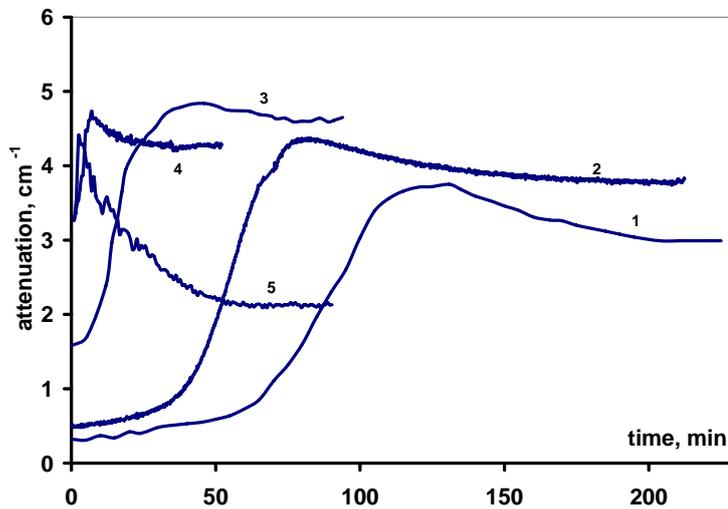
Figure 2. Changes in sound attenuation during adhesive cure at different temperatures. Notes are the same as in Fig. 1.
