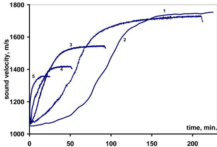
Figure 1. Changes in longitudinal sound velocity during epoxy adhesive cure at different temperatures. 1-100<sup>0</sup>C, 2-120<sup>0</sup>C, 3-140<sup>0</sup>C, 4-160<sup>0</sup>C, 5- 180<sup>0</sup>C.
