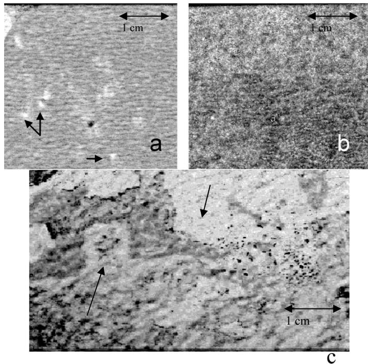
Figure 7. Acoustic C-scans images of the adhesive/metal interface (a and c) and bulk adhesive microstructure (b) obtained at a frequency of 50 MHz. Specimens were exposed to the high humidity and slightly elevated temperatures (70°C).
