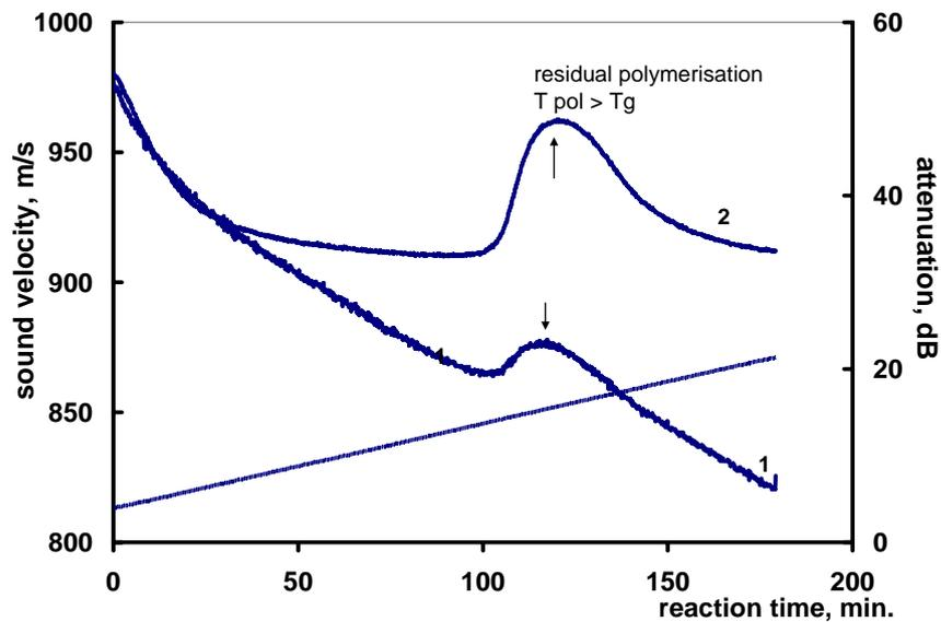
Figure 4. Changes of sound velocity (1) and attenuation (2) during non-isothermal cure. Straight line shows temperature profile. Heating rate is  $1^{\circ}\text{C}/\text{min}$ .
