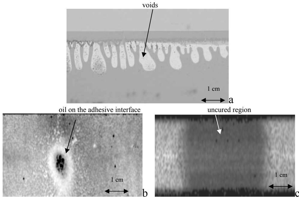
Figure 6. Acoustic C-scans illustrate the three types of adhesive joint defects. a-voids in the adhesive layer; b- adhesive problems on the metal/adhesive interface caused by oil presence; c-cohesion defects caused by improper cure. Images are obtained using 50 MHz spherical acoustic lens. Specimens consist of two steel sheets with a thickness of 0.8 mm, joined by a 0.3 mm layer of some industrial structural epoxy adhesive.
