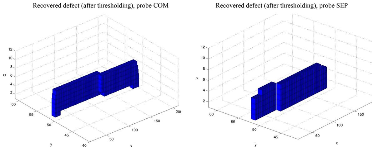
**Figure 7** 3D reconstruction results on a 3 mm depth crack for COM probe (left hand side) and SEP probe (right hand side). The estimated depth are about 3mm for the COM probe, and 2.5 mm for the SEP probe.
