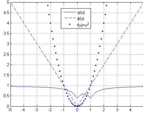
Figure 2 Shape of penalization functions  $\phi(u)$  and  $\psi(u)$  used.
