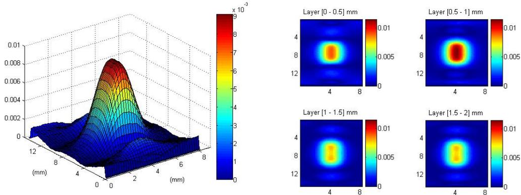
**Figure 5 SEP probe: PSF.** Left hand side: 3D shape of the modulus of the PSF first layer, Right hand side: 2D modulus of the PSF from first ([0-0.5] mm) to fourth layer ([1.5-2] mm)
