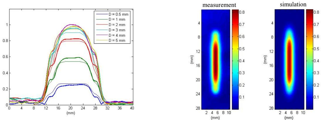
**Figure 4 COM probe: Comparison between real and synthesized data.** Left hand side: longitudinal cross-section of real (bold line) and synthesized data (normal line) along the 15 mm notches. Right hand side: modulus of the real data (left hand side) and the synthesized data (right hand side) for the 2mm depth, 15 mm long, 0.2 mm width notch
