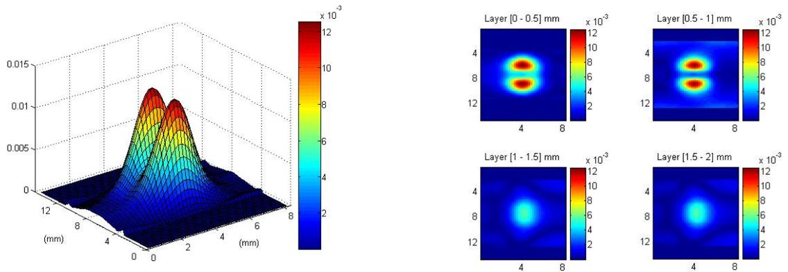
**Figure 3 COM probe: PSF.** Left hand side: 3D shape of the modulus of the PSF first layer, Right hand side: 2D modulus of the PSF from first ([0-0.5] mm) to fourth layer ([1.5-2] mm)
