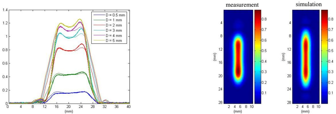
**Figure 6 SEP probe: Comparison between real and synthesized data.** Left hand side: longitudinal cross-section of real (bold line) and synthesized data (normal line) along the 15 mm notches. Right hand side: modulus of the real data (left hand side) and the synthesized data (right hand side) for the 2mm depth, 15 mm long, 0.2 mm width notch
