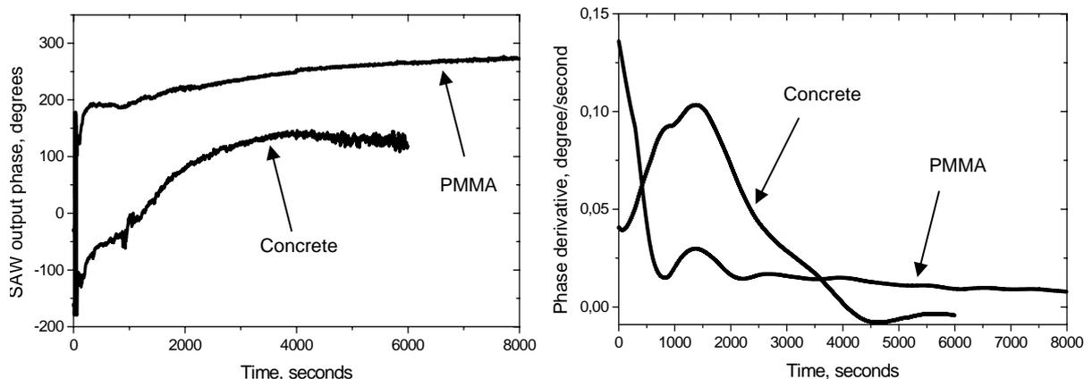
Figure 8. AC-SAW monitoring of drying paint: output phase (left) and its derivative (right) variations in time.
