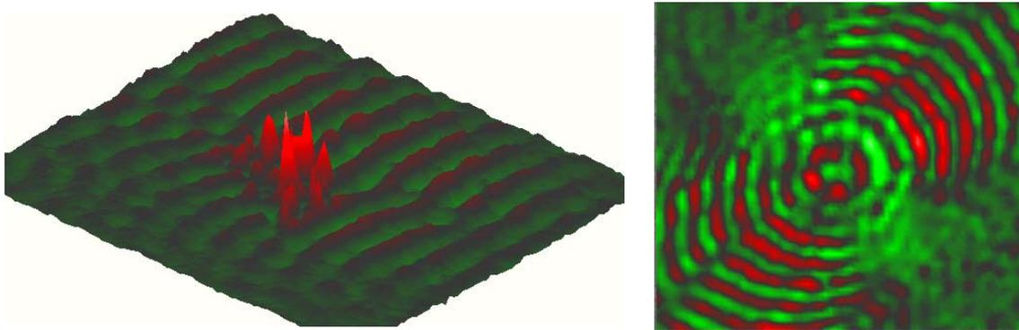
Figure 9. Material inspection in WIM: AC-PAW scattering by an impact in CFR-composite (left); anisotropy of PAW propagation in beech veneer (right).
