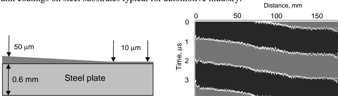
Figure 7. FSTM-profilometry: (left) configuration of paint coating; (right) FSTM-B-scan (white lines indicate positions of zero displacements).
