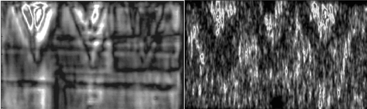
Figure 5. AC-plate wave imaging of simulated delaminations in honeycomb liners: front (left) and reverse (right) sides. Sample kindly provided by GROB Aerospace/Mindelheim-Mattsies.
