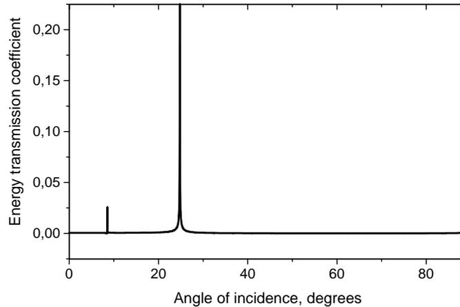
Figure 1. Transmission coefficient as a function of angle of incidence for a 0.5 mm PMMA plate in air (frequency  $f = 450 \text{ kHz}$ ).
