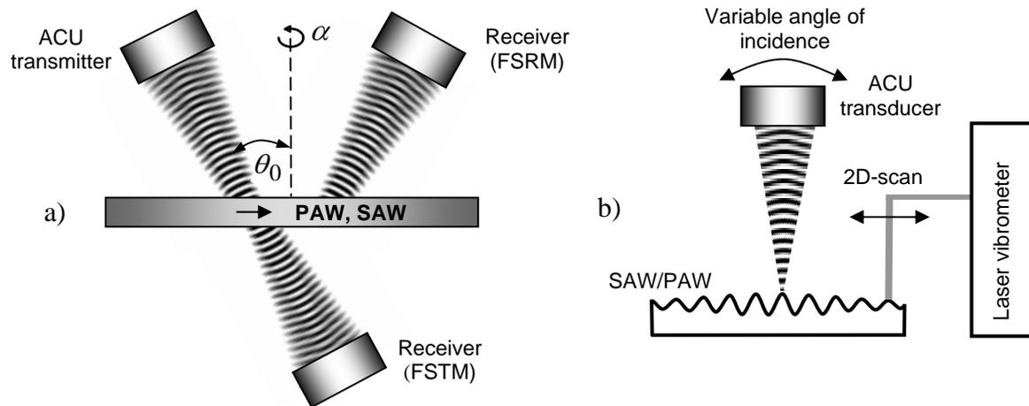
Figures 4 a, b. FSTM- and FSRM-configurations of ACU conversion (a); wave form imaging set-up (b).
