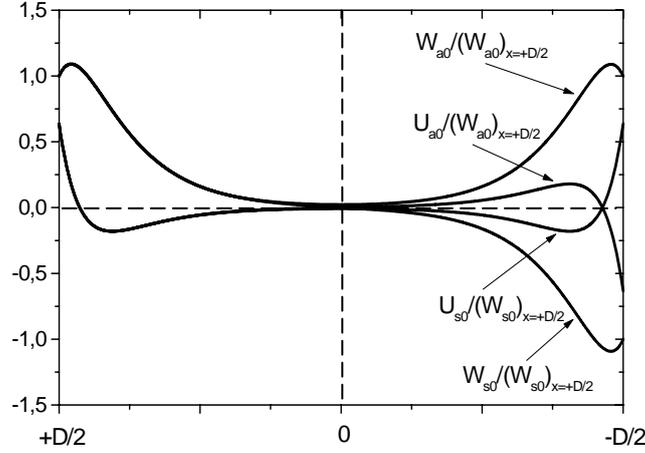
Figure 2. Depth distributions of normalized displacements of zero-order modes in PMMA plate at  $k_t D = 30$ .
