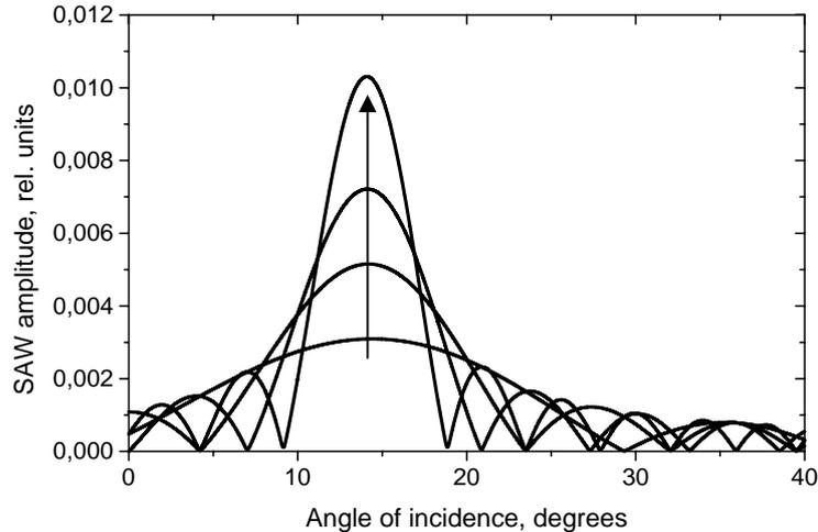
Figure 3. Calculated efficiency of ACU-SAW conversion in PMMA as a function of angle of incidence for different values of aperture ( $W$ ) of 400-kHz-ACU-beam. The arrow corresponds to  $W = 3, 5, 7, \text{ and } 10$  mm.
