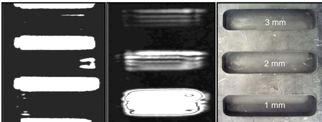
Figure 6. Single-sided scans of hidden cavities in Al-sample (right): AC-SAW (left) and AC-PAW (middle).
