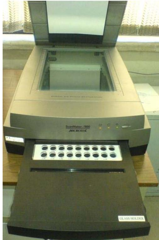
Fig. 1 The film scanner with a calibration film
