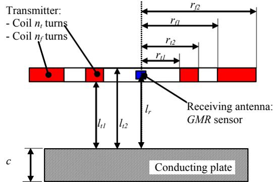
**Table 1.** Dimensions of transmitter-receiver system as used in calculations and/or measurements.
