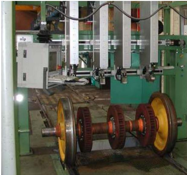
Fig. 7 Wheel set test system (DB)
