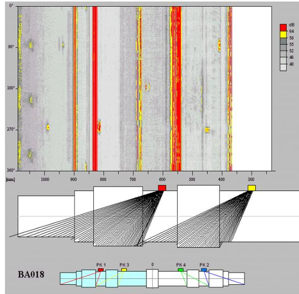
Fig. 8 Test result of the wheel set (left side)
