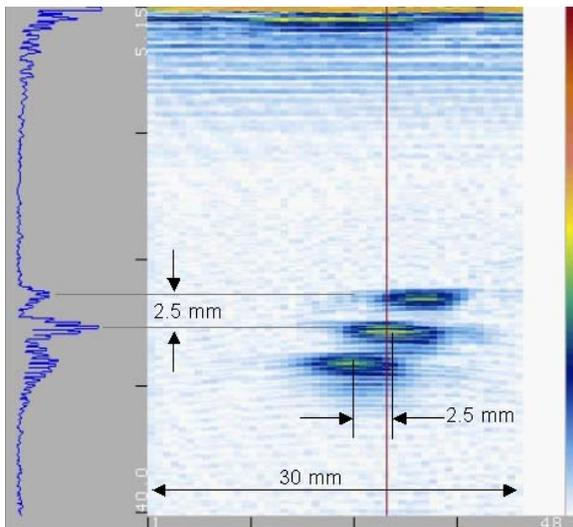
Fig. 10 B-scan of 3 SDH (1mm diameter)
