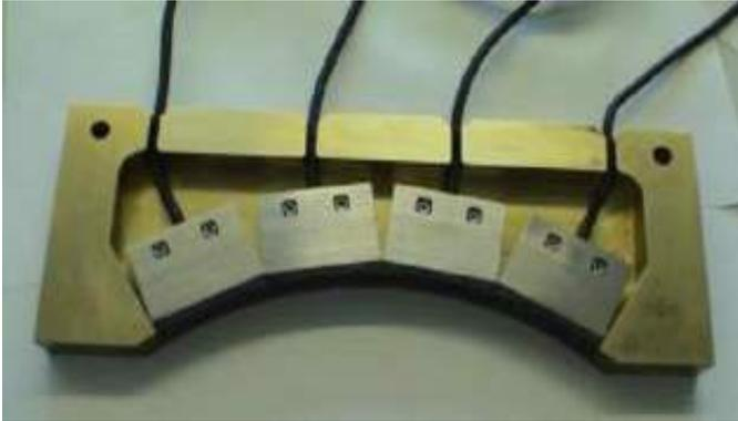
Fig. 3 ROWA probe (4x32 elements)
