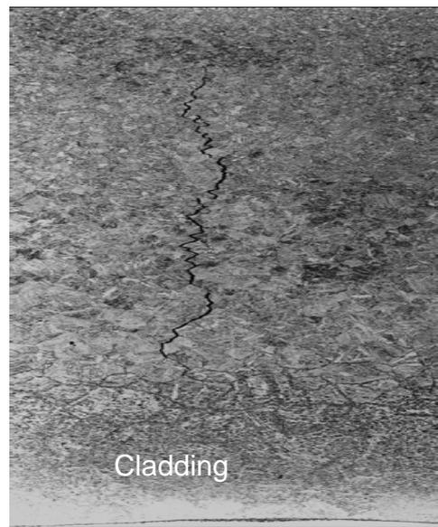
Fig. 2: Underclad crack, 4 mm deep
