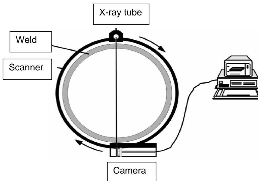
Fig.3: Radiometric weld inspection system "Tomocar"
