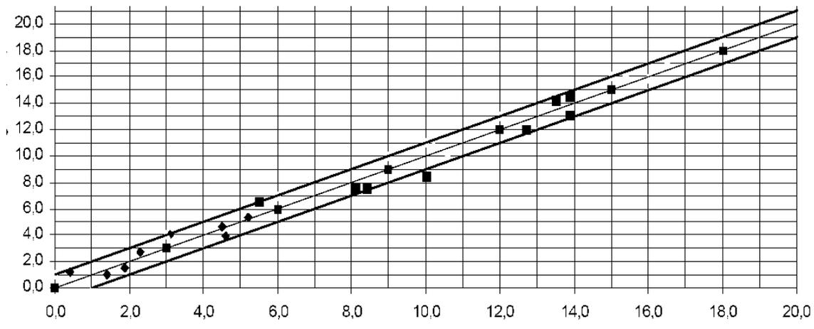
Fig.4: Sizing results (metallography vs. tomography); data from wall thickness, flaw depth and flaw size (mm)
