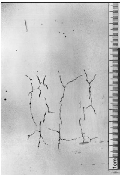
Fig.1: IGSCC field in the cladding
