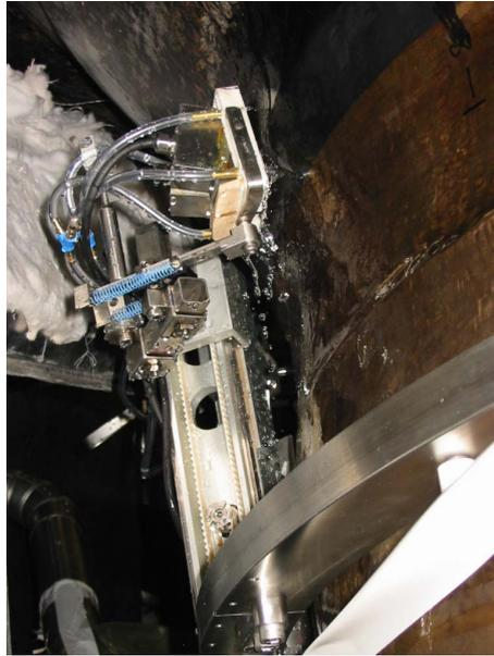
Figure 12: TRL PA probe on MCP weld
