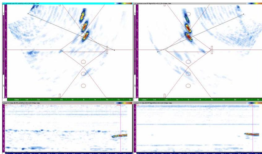
Figure 10: image of one-line scan with TRL PA probes
