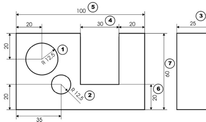
**Fig. 3** Measures of the alloy test object. The seven measurements performed with the fitted geometries are marked with encircled numbers.
