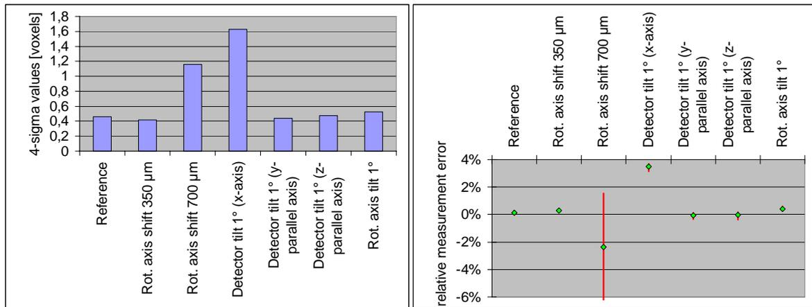
**Fig. 6** Measurement quality according to the 4-sigma values (left) and relative measurement errors (right) for different geometry misalignments, along with the reference case with accurate alignment.
