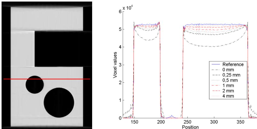
**Fig. 5** Voxel value profiles in the reconstructed volume (right) along the marked line (left) for different source prefiltrations.
