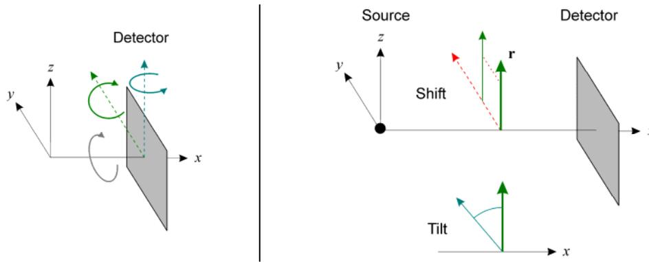
**Fig. 2** Misalignments of the detector (left) and of the object rotation axis (right).
