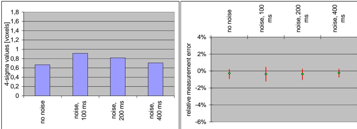
**Fig. 8** Measurement quality according to the 4-sigma values (left) and relative measurement errors (right) for different detector exposure times, along with the reference case without quantum noise.
