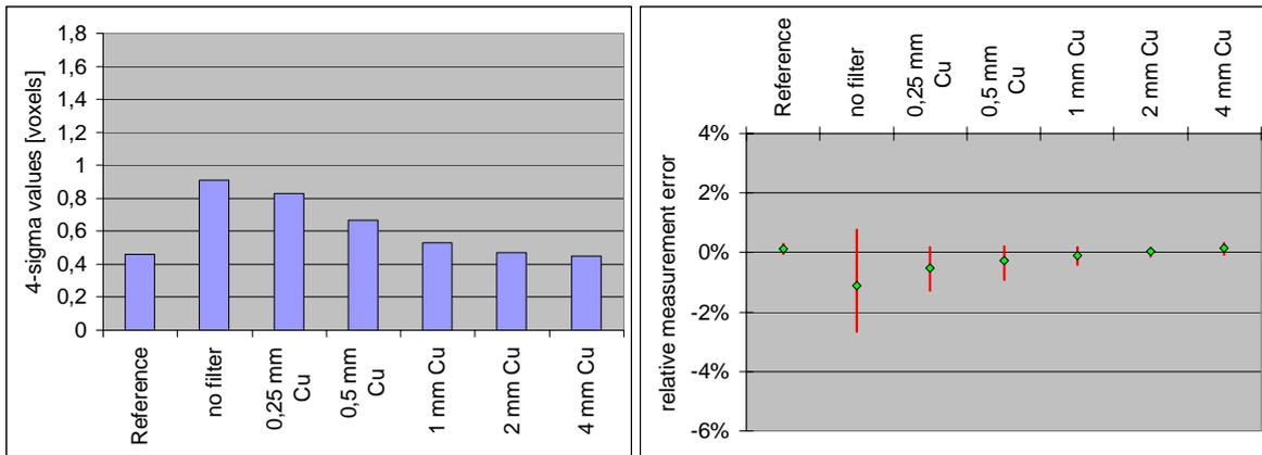
**Fig. 4** Measurement quality according to the 4-sigma values (left) and relative measurement errors (right) for different source prefiltration, along with the monochromatic reference case.
