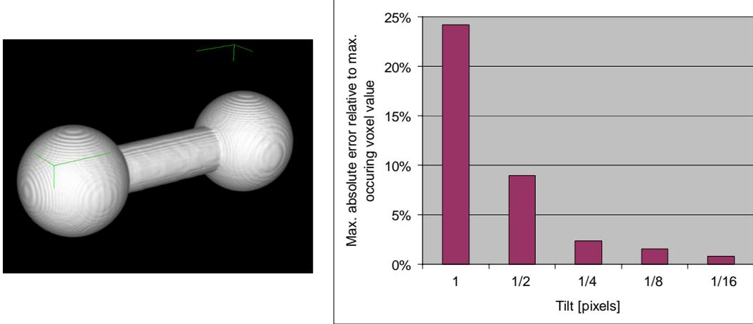
**Fig. 7** Object for investigation of the maximum tolerable detector rotation around the x-axis (left). The maximum of the absolute error relative to the maximum of the occurring voxel values is shown on the right for different detector tilts.
