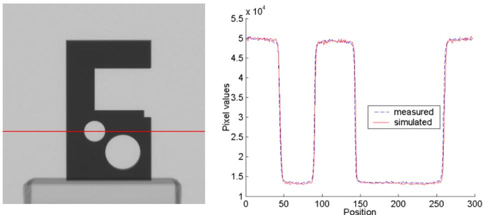
**Fig. 1** Comparison of measured and simulated X-ray projection pixel values.
