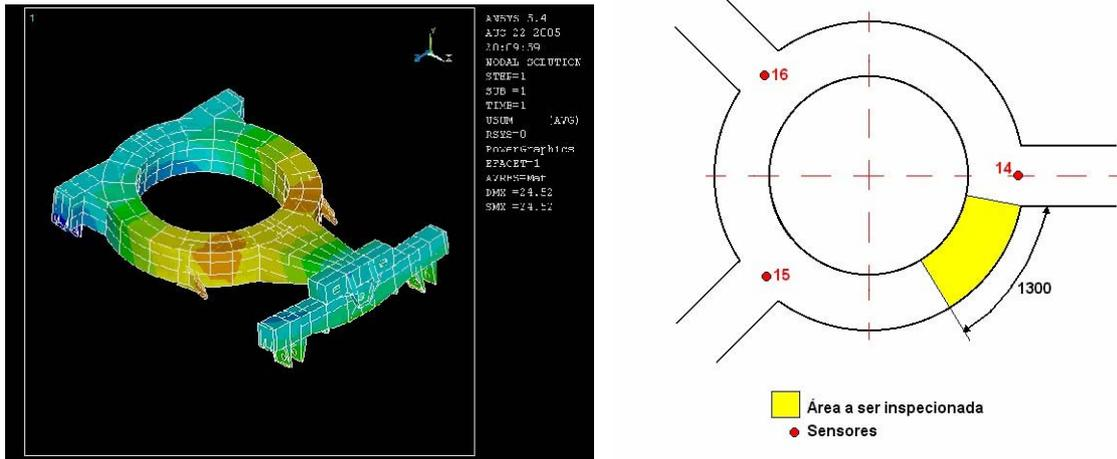
**Figure 5.** Top: result of a finite element analysis. Bottom: result of acoustic emission.
