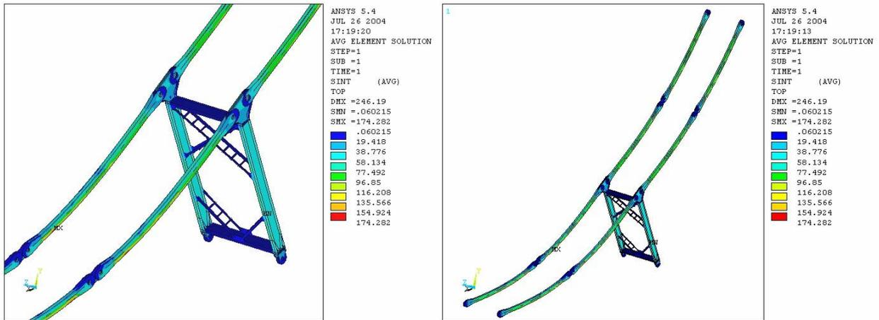
**Figure 7.** Finite element stress analysis in tie rods
