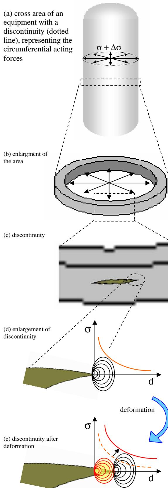
**Figure 1.** (a), (b) e (c) amplified image of the region where the discontinuity is located; (d) region of stress concentration at the tip of the discontinuity; (e) displacement of stress versus position after propagation of size.
