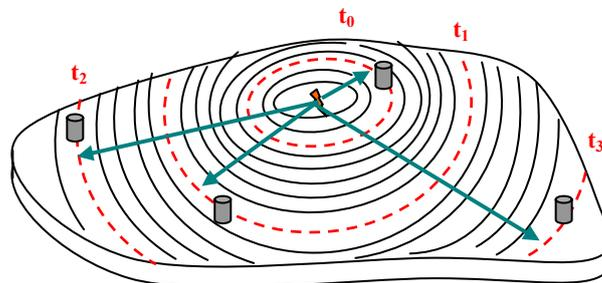
**Figure 2.** Location principle drawing. Two parameters are need: sound speed of material and arrival time for each sensor.
