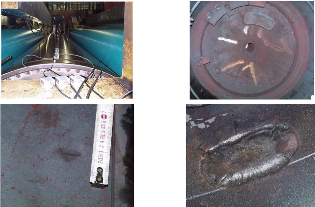
**Figure 3:** AT on drying cylinders (steam drums) in paper mills. Application of sensors on cylindrical shell (top left) and defects found at follow-up inside inspections: casting defect (top right), crack like defect (bottom left) and erosion (bottom right).
