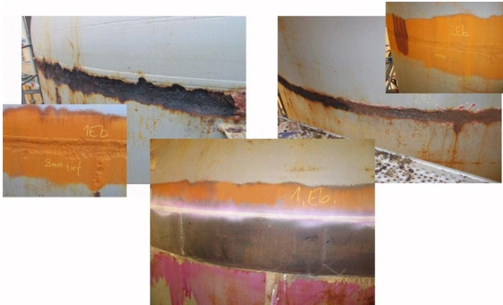
**Figure 7:** Follow-up NDT to the AT indications and performed repair, top left side photo - corrosion damage with depth up to 8 mm near to circular weld seam of the upper head, top right side photo – next corrosion damage near to structural ring element of thermal insulation with depth up to 7 mm, photo at bottom – repair of corrosion damage with reinforcing segments.
