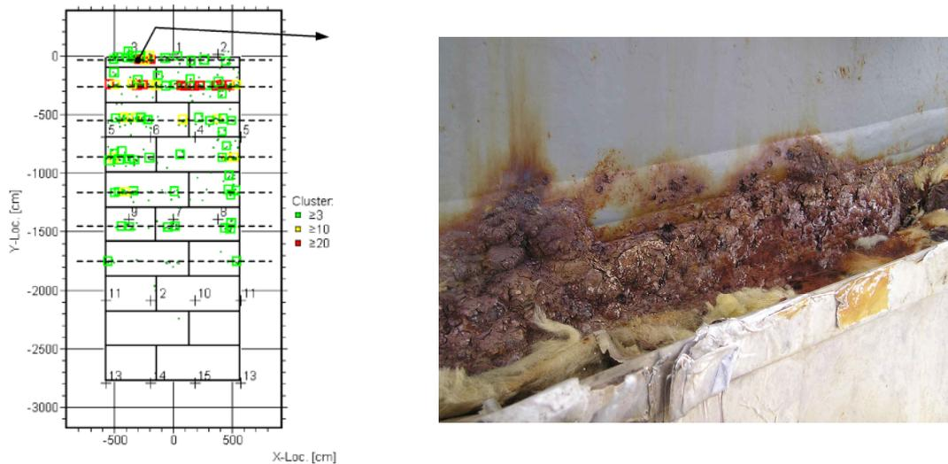
**Figure 6:** Preliminary location result just after the test and visually detected finding at one suspicious area, sketch on the left – unwrapped cylindrical shell with linear aligned clusters of located events at different vertical levels indicated by dash lines, photo on the right – taken after removal of thermal insulation at position indicated in the left sketch by an arrowed line with dot at its origin.
