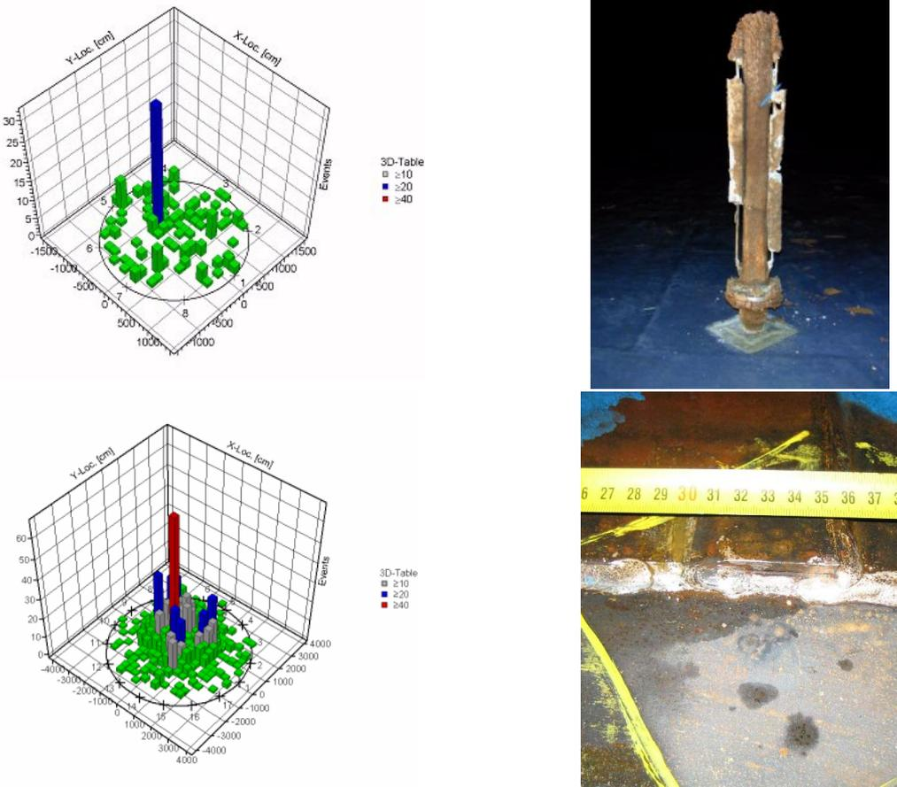
**Figure 5:** AT on flat bottomed storage tanks for corrosion and leakage. Evaluation of a test on a salt water tank (top left) and found sacrificial anode (top right). Evaluation of a test on a crude oil tank filled with water for strength test (bottom left) and found improper welding at an overlap (bottom right).
