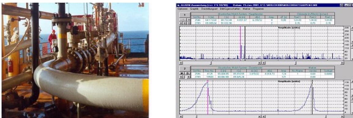
**Figure 4:** Leak detection with the ALARM tool employed at a 360 km off-shore pipeline (left) and evaluation of the pig run (right). One can easily see two peaks in the plot at the bottom indicating two different leaks.
