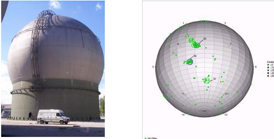
**Figure 2:** AT on storage spheres. Repetition test of natural gas storage sphere (left) and found indications of defects by AT (right)
