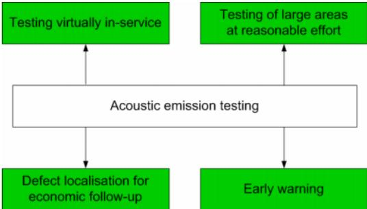
**Figure 1:** Main advantages of acoustic emission testing for industrial applications.
