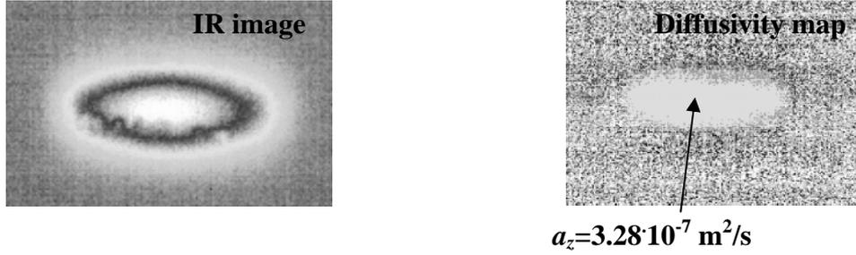
**Fig. 1.** Converting the  $R$ -surface IR image sequence into the diffusivity map (ThermoFit Pro program, Innovation Ltd, Russia)
