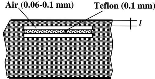
**Fig. 5.** The model of defects in a graphite/epoxy composite (Teflon inserts surrounded by air gaps)
