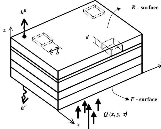
Fig. 3. 3D modeling of defects in graphite/epoxy composite
