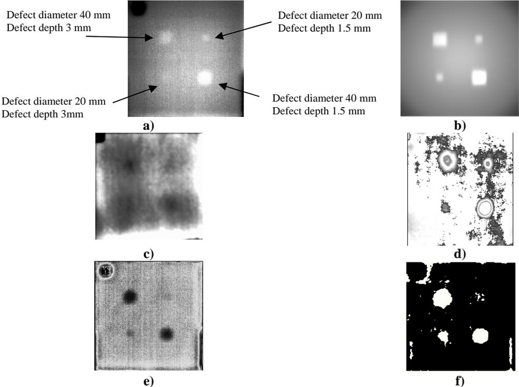
**Fig. 4.** Thermal NDT of a 15-mm thick graphite/epoxy sample (10 s heating):
