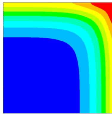
**Figure 9:** Calculated temperature distribution for the same case as shown in Figure 8, but after a heating period of 0.4 sec.
