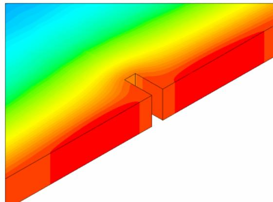
**Figure 15:** Calculated temperature distribution for the same case as shown in Figure 14, but after a heating period of 0.4 sec.
