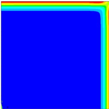
**Figure 8:** Calculated temperature distribution in one corner of a square after 0.01sec inductive heating, the penetration depth of the eddy current is 1mm. The size of the shown area is 15x15mm.
