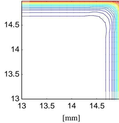
**Figure 7:** Calculated streamlines in the corner of a workpiece (penetration depth of the eddy current is 0.1mm)
