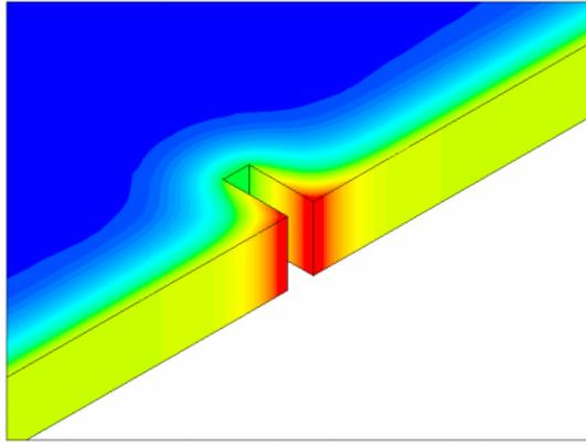
**Figure 16:** Calculated temperature distribution around a surface crack with a depth of 1mm after 0.01sec inductive heating. The penetration depth of the eddy current is 0.1mm.
