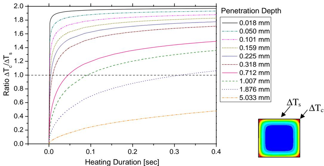
**Figure 11:** Ratio between the temperature increase in the corner and at the side of the square as a function of the heating period for different penetration depth values. The insert shows the definition of the temperatures.
