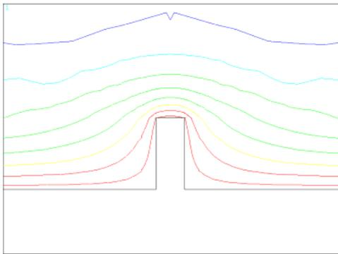
**Figure 12:** Calculated streamlines around a surface crack with a depth of 1mm (penetration depth of the eddy current is 1mm)
