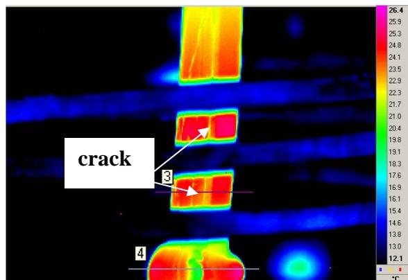
**Figure 3:** Infrared image of the heated stainless steel wire.
