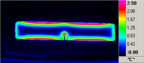
**Figure 5:** Infrared image of the heated steel sheet with an artificial crack
