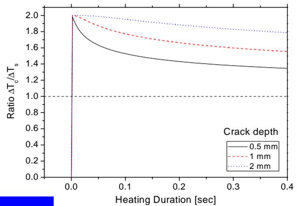
**Figure 18:** Ratio between the temperature increase in the corner of the crack and at the side of the sample as a function of the heating period for different crack depth values. The curves are calculated with the analytical model of [7,8].
