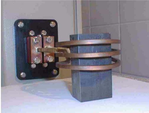
**Figure 1:** Inductive heating of a steel workpiece inserted into the induction coil.
