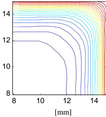
**Figure 6:** Calculated streamlines in the corner of a workpiece (penetration depth of the eddy current is 1mm)
