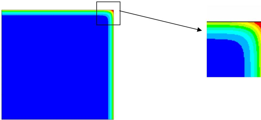
**Figure 10:** Calculated temperature distribution in a corner of a square after 0.01sec inductive heating, with a penetration depth of the eddy current of 0.1mm. The size of the shown area is 15x15mm. At the right side of the figure the temperature distribution in the corner is shown enlarged.
