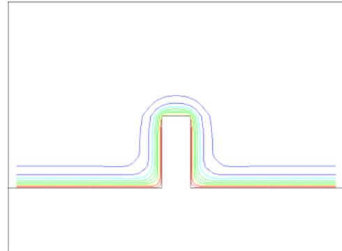
**Figure 13:** Calculated streamlines around a surface crack with a depth of 1mm (penetration depth of the eddy current is 0.1mm)
