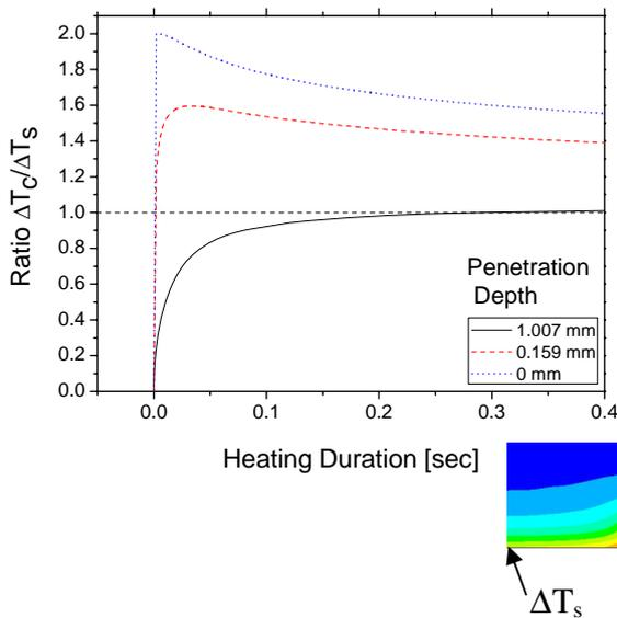
**Figure 17:** Ratio between the temperature increase in the corner of the crack and at the side of the sample as a function of the heating period for different penetration depth values. The insert shows the definition of the temperatures.
