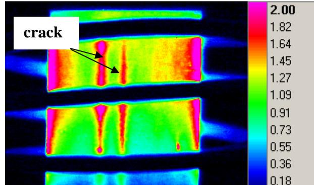
**Figure 2:** Infrared image of the heated steel shown in Figure 1.
