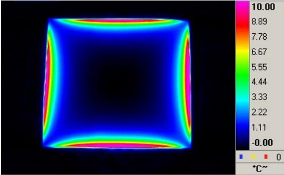
**Figure 4:** Infrared image of the heated steel sheet which forms a square
