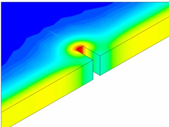
**Figure 14:** Calculated temperature distribution around a surface crack with a depth of 1mm after 0.01sec inductive heating. The penetration depth of the eddy current is 1mm.
