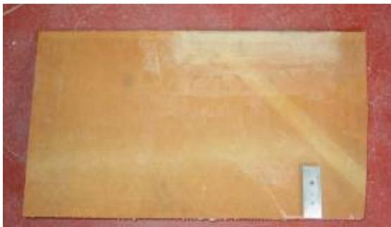
Figure 2 Left: composite part with hole type IQI
