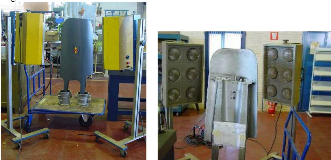
Figure 5 : Set up used for infrared testing of composite speedbrakes (front and rear view showing  $2 \times 6$  halogen lamps used to generate the thermal pulse)
