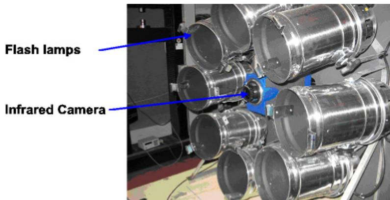
Figure 3. Set of flash lamps producing modulated thermal wave.
