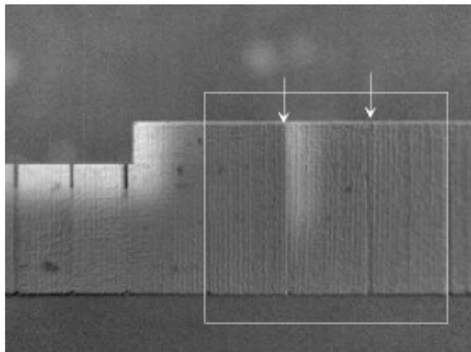
Figure 4. LOCKIN images of a W7X target element.
