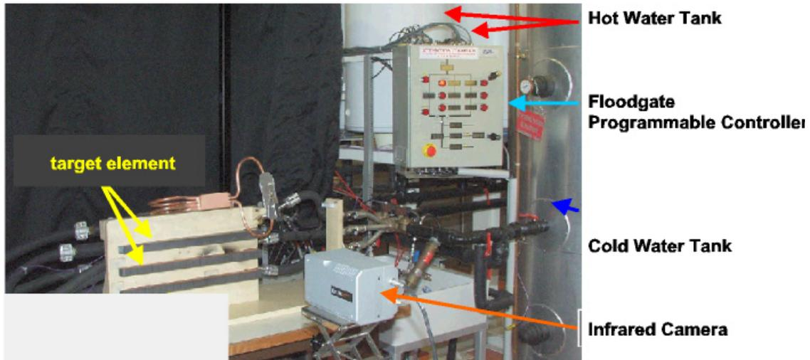
Figure 2. SATIR bench : experimental set-up
