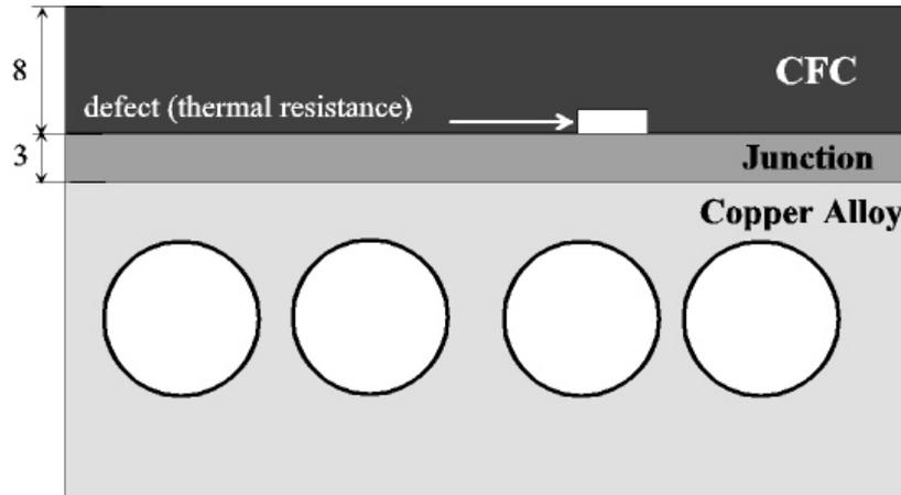
Figure 1. Simplified drawing of a section of the W7X target element and a defect.
