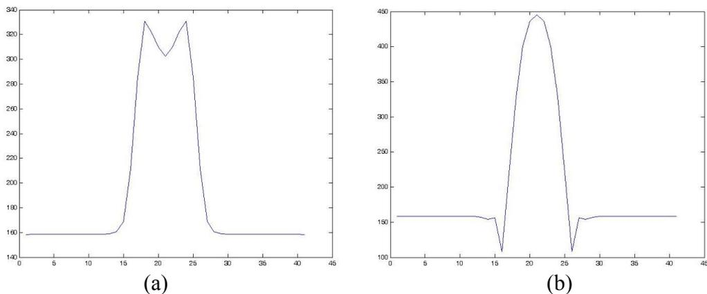
Fig. 5 Frequency response to (a) an air hole (b) a conductive sphere in the dielectric
