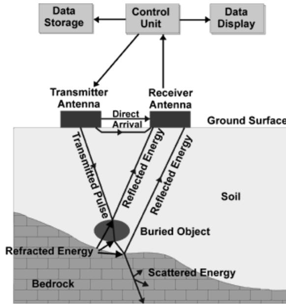
Fig. 1 Geometry of the GPR system
