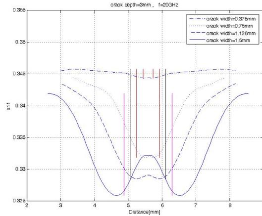
Fig. 7 Effect of crack width
