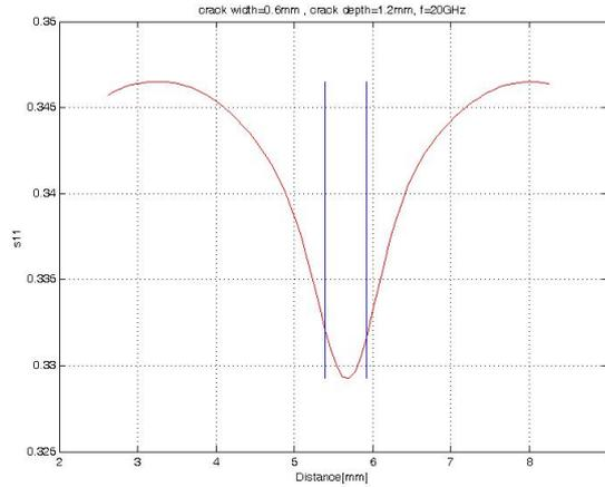
Fig. 4 Reflect coefficient changing over a surface cracked metal
