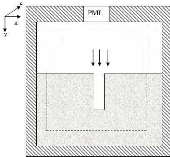
Fig. 2 FDTD simulation of the cracked surface
