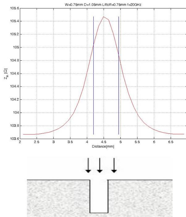
Fig. 3 Antenna impedance changing over a surface cracked metal
