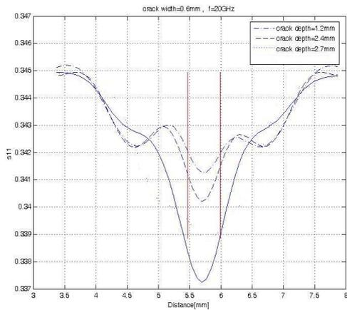
Fig. 6 Effect of crack depth
