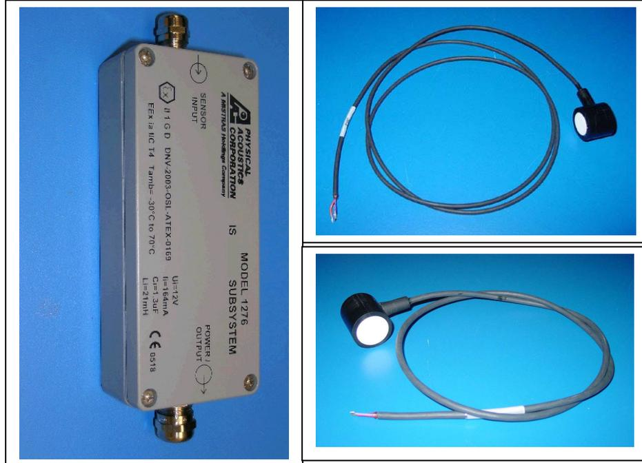
**Figure 2:** Acoustic Emission sensors, I.S. unit top right is used with the I.S. pre-amplifier (left), the larger sensor has a built in pulser and pre-amplifier to drive >500m of cable. All are IP66 rated.
