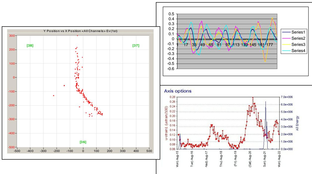
**Figure 5:** Top left; Acoustic emission locations, the green numbers are sensor positions, red dots are the source positions, X,Y scale in mm. Top right; high speed strain transient at four gauges resulting from wave impact (20 seconds time scale). Bottom right; Peak hourly strain acquired over a seven day period.
