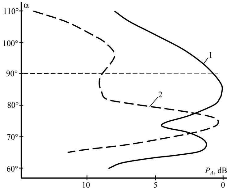
**Fig.3.** Acoustical field of *STV* probe with operating frequency 1 MHz (1) and 1,85 MHz (2).
