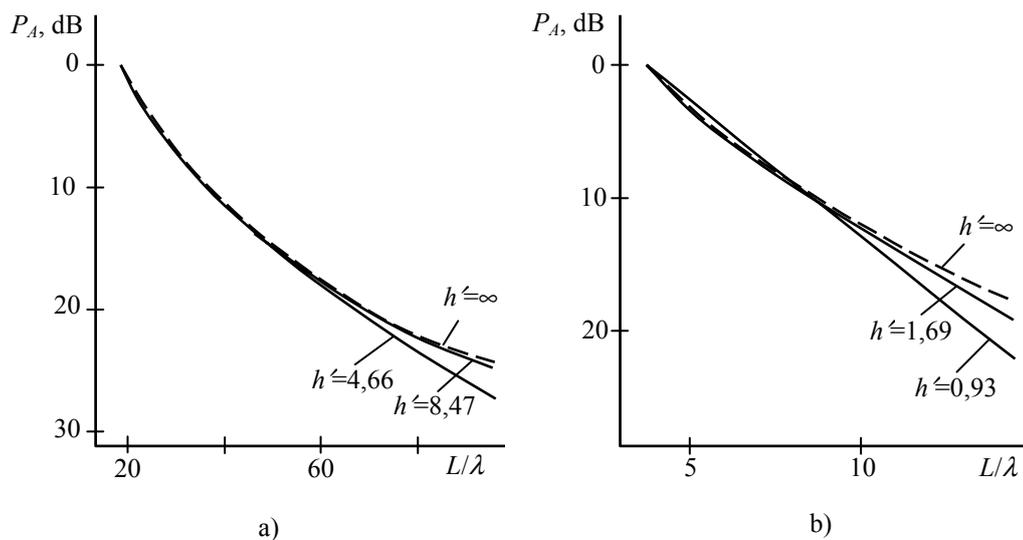
**Fig.6.** Normalized experimental dependencies  $P_A(L/\lambda)$  for steel plates of different thickness for  $v = 1$  MHz (a) and  $5$  MHz (b).
