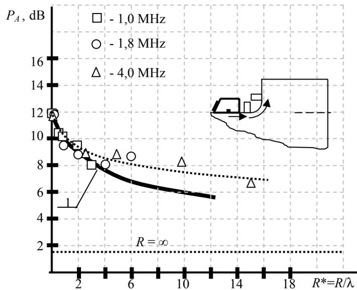
**Fig.4.** Amplitude  $P_A$  of Rayleigh wave transmitted through curvilinear surface (1) and maximum of *STV* amplitude, transformed at the fillet transition (2).
