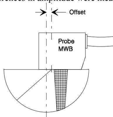
Direct contact test on 25mm half - cylinder sample
