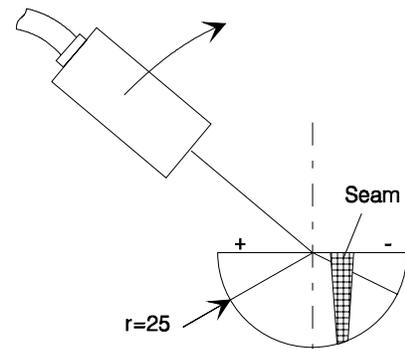
Half - cylinder arrangement for the determination of sound velocities
