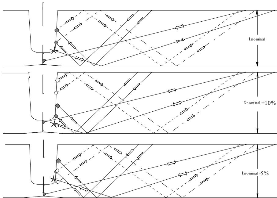
Figure 2: Variations of sound paths for different wall thickness
