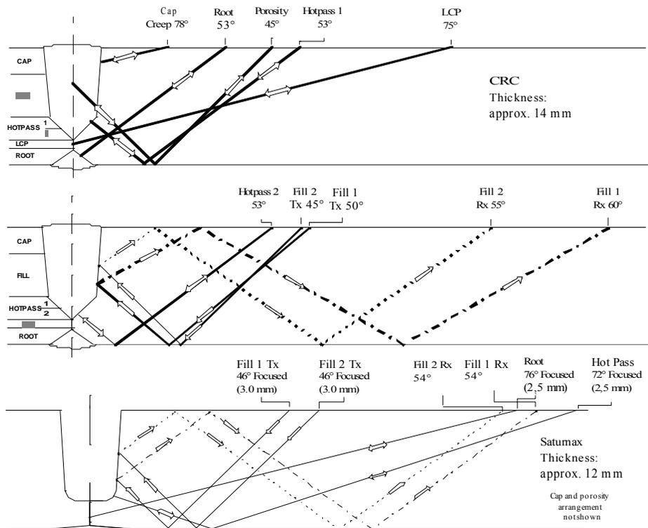
Figure 1: Schematic showing transducer placement, sound paths and target positions on welds
