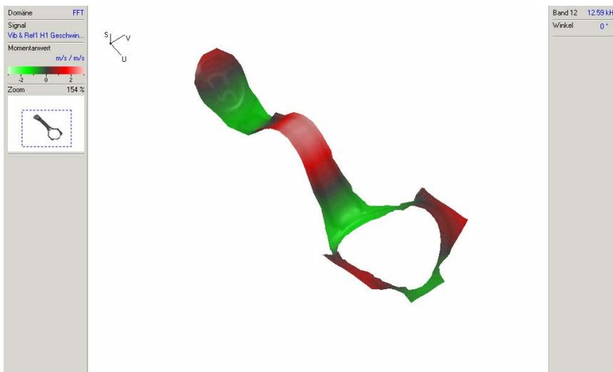
**Figure 9:** 3-D view of a conrod at 12590 Hz
