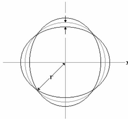
**Figure 3:** Schematic view of a transversal vibration in ring level
