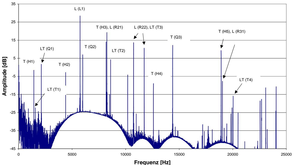
**Figure 10:** Microphone spectrum of a conrod (far field)
