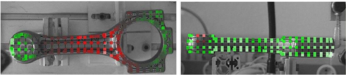
**Figure 8:** Laser scan of conrods (green: low vibration red: high vibration)
