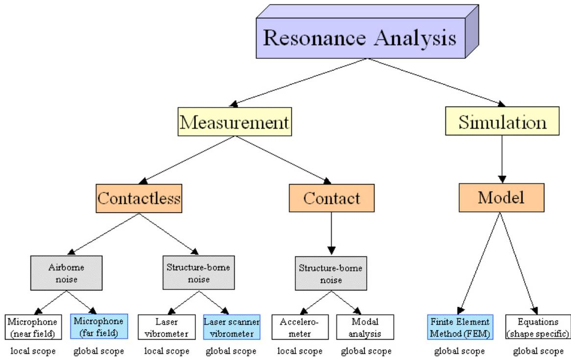
**Figure 1:** Methods for the determination of resonance frequencies
