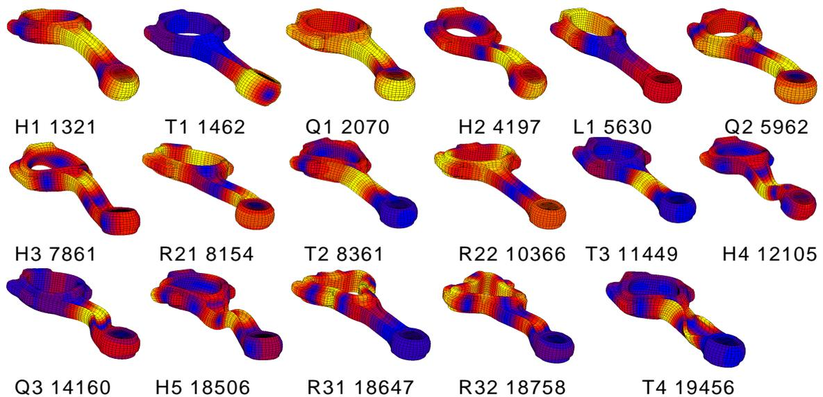
**Figure 7:** FEM of a conrod up to 20 kHz (colours: light is high amplitude, dark is low amplitude. Denotation: the alphanumeric is the mode (see below), the following number the frequency)
