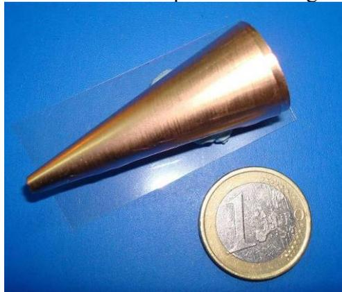
Figure 3. Conical Swiss roll made from LONGLITETM200
