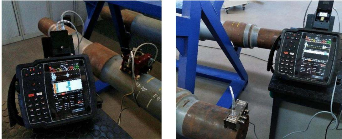
Figure 4. Axle inspection with Innerspec PowerBox H using a) 274A0093-M00 sensor b) 274A0244 sensor
