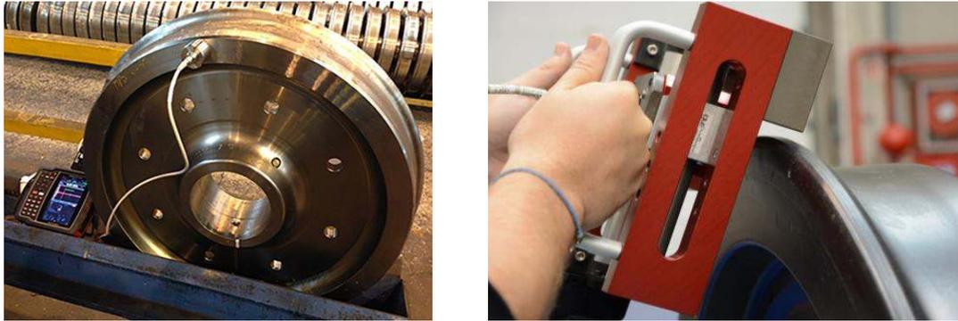
Figure 2. Innerspec PowerBox H performing Stress Measurement on rail wheel a) without positioner b) with positioner
