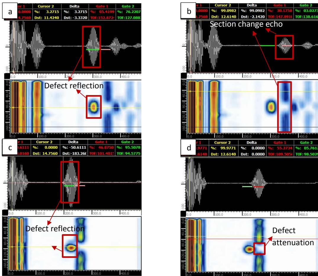
Figure 5. Rail axle inspection results a) 274A0093-M00 sensor with defect b) 274A0093-M00 without sensor defect c) 274A0244 sensor with defect d) 274A0244 sensor without defect
