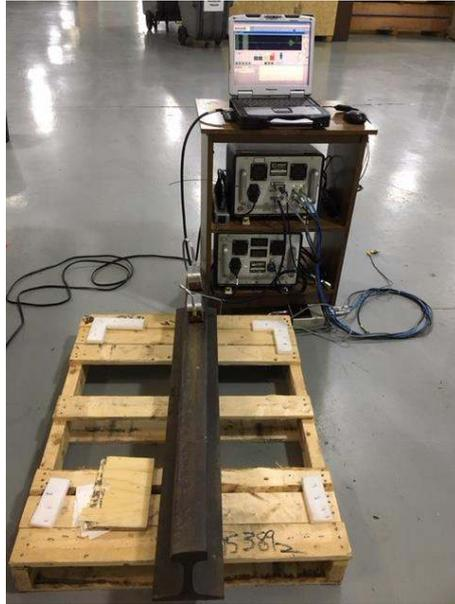
**Figure 6. Laboratory setup working in Pitch Catch configuration using Innerspec PowerBox 2**
