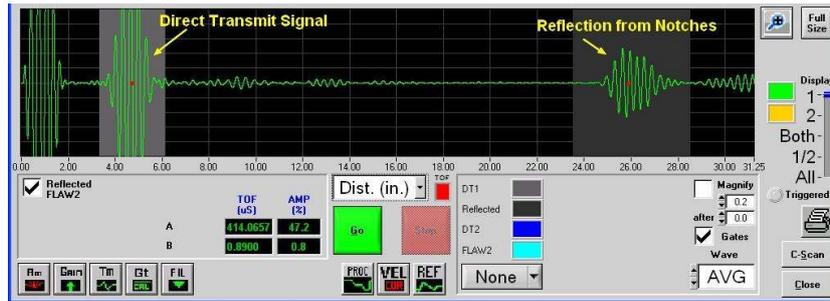
Figure 7. Reflection from Rail Head notch in Pitch - Catch mode. A-Scan View
