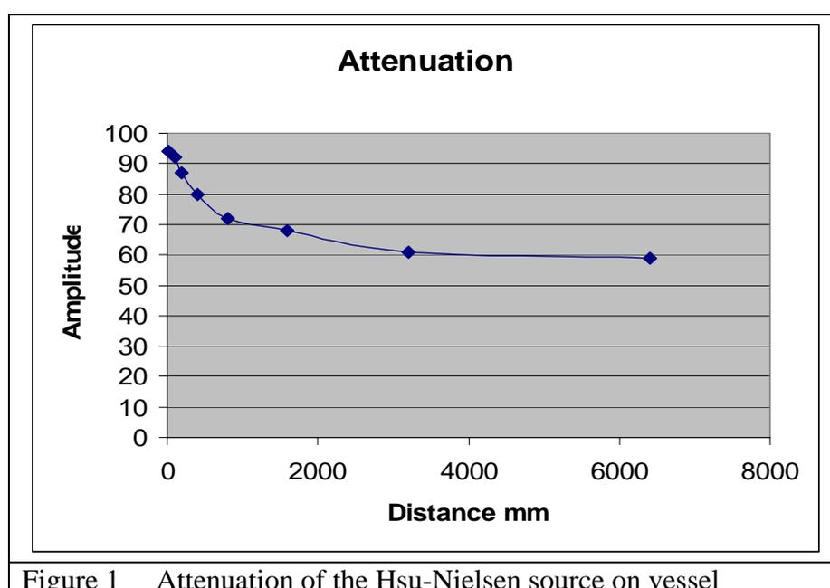
Figure 1 Attenuation of the Hsu-Nielsen source on vessel
