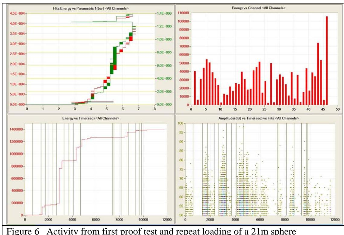
Figure 6 Activity from first proof test and repeat loading of a 21m sphere
