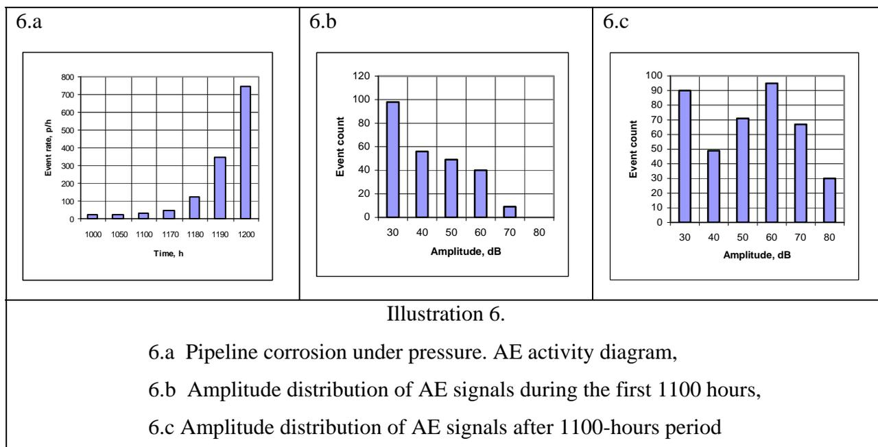
During the period between 500 and 900 hours AE activity remained constant. After 1150-hours period activity began to increase drastically and totaled 750 pulse/hour (Illustration 6.a), which is an evidence of drastic speed growth in corrosion destruction. Analysis of
